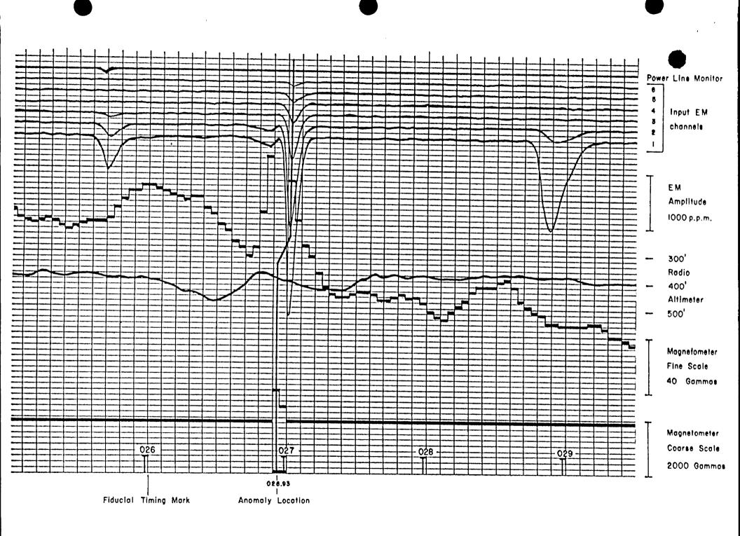
Representative INPUT, Magnetometer and Altimeter Recording
