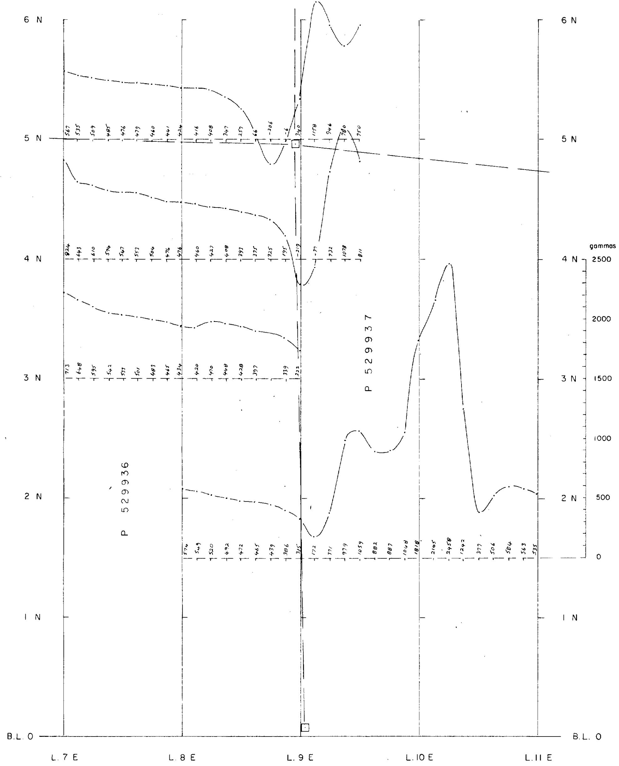
Instrumentation : Geometrics G 816 magnetometer
