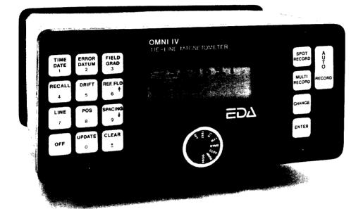
Four Magnetometers in One Self Correcting for Diurnal Variations Reduced Instrumentation Requirements 25% Weight Reduction User Friendly Keypad Operation Universal Computer Interface Comprehensive Software Packages
