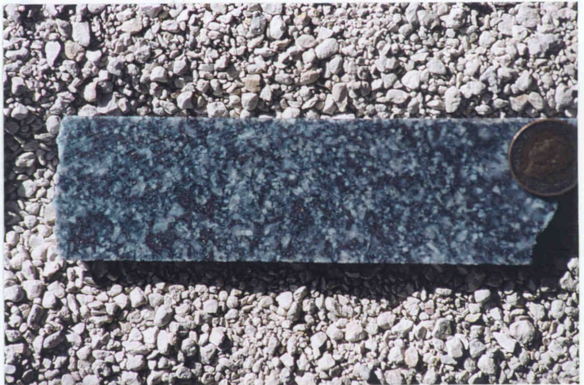
Photograph 5. Sample (123.3 - 123.42 m) of the medium to coarse grained, leucoxene-bearing leucogabbro containing 12-15% interstitial, moderately magnetic pyrrhotite, minor pyrite and very minor traces of chalcopyrite.
