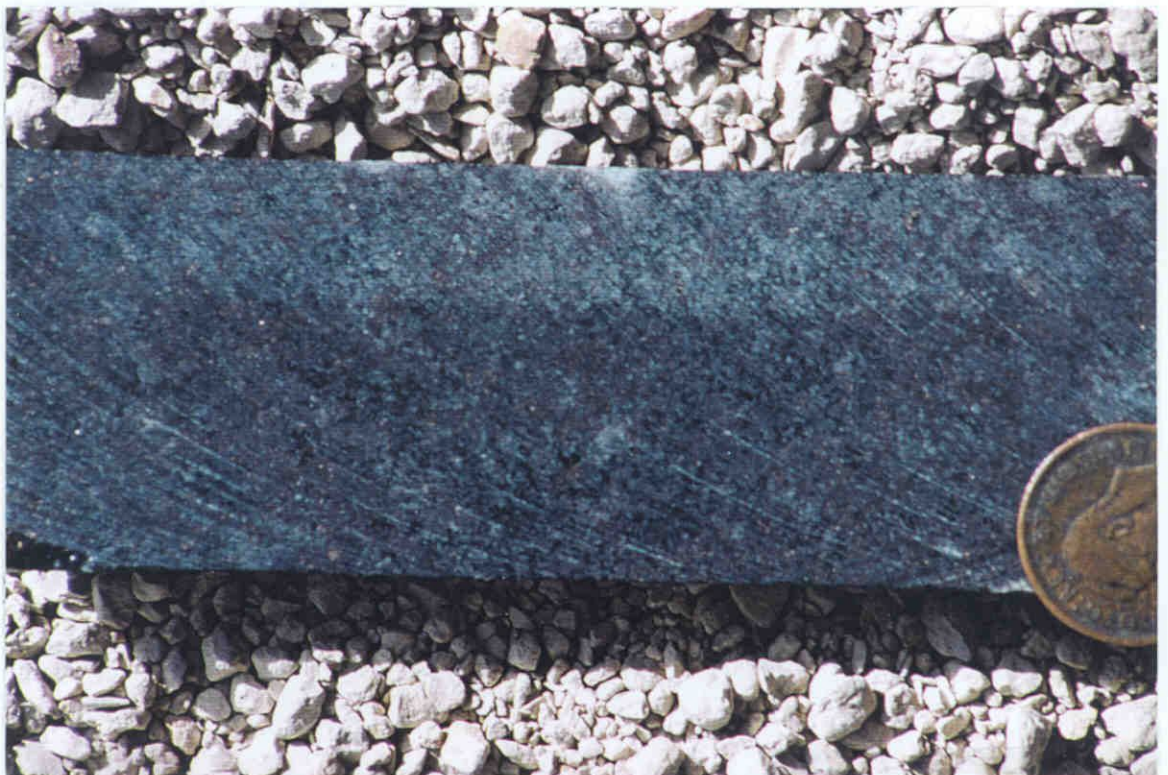
Photograph 7. Medium grained, highly serpentinized olivine-bearing pyroxenite (137.65 - 137.75 m) from the main sulphide horizon. The sample contains 15-20% interstitial fine grained pyrrhotite, minor pyrite and trace chalcopyrite.
