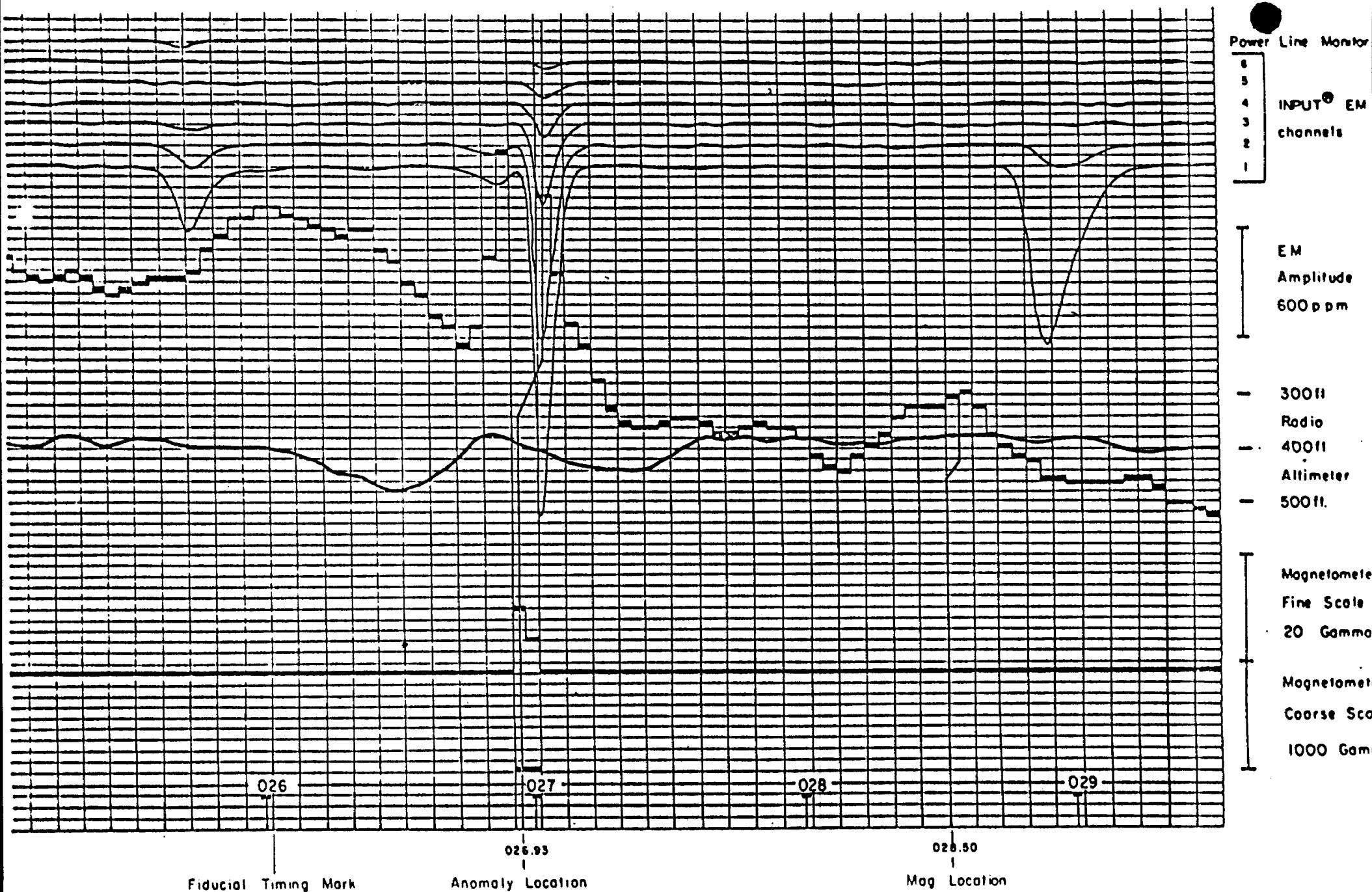
Representative INPUT®, Magnetometer and Altimeter Recording
