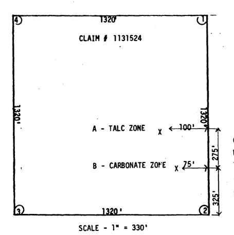
TRENCH APPROX.250'LONG BY 10'WIDE VISABLE TALC THROUGHOUT THE TRENCH WITH GRADES OF UP TO 95% PURE. SIX PLUGGER HOLES WHERE PUT INTO THIS ZONE AND BLASTED, SAMPLES WHERE GIVEN TO LUZENAC INC. AND THE GRADE WAS 90 - 95% AS INDICATED ABOVE. TO THE WEST OF THIS TRENCH APPROX. 300' IS A OUTCROP WITH THE SAME GRADE UNCOVERED GREEN CARBONATE ZONE WITH QUARTZ STRINGERS. HAND TOOLS, PLUGGER WORK AND BLASTED EIGHT SAMPLES FROM THIS ZONE RETURNEE
