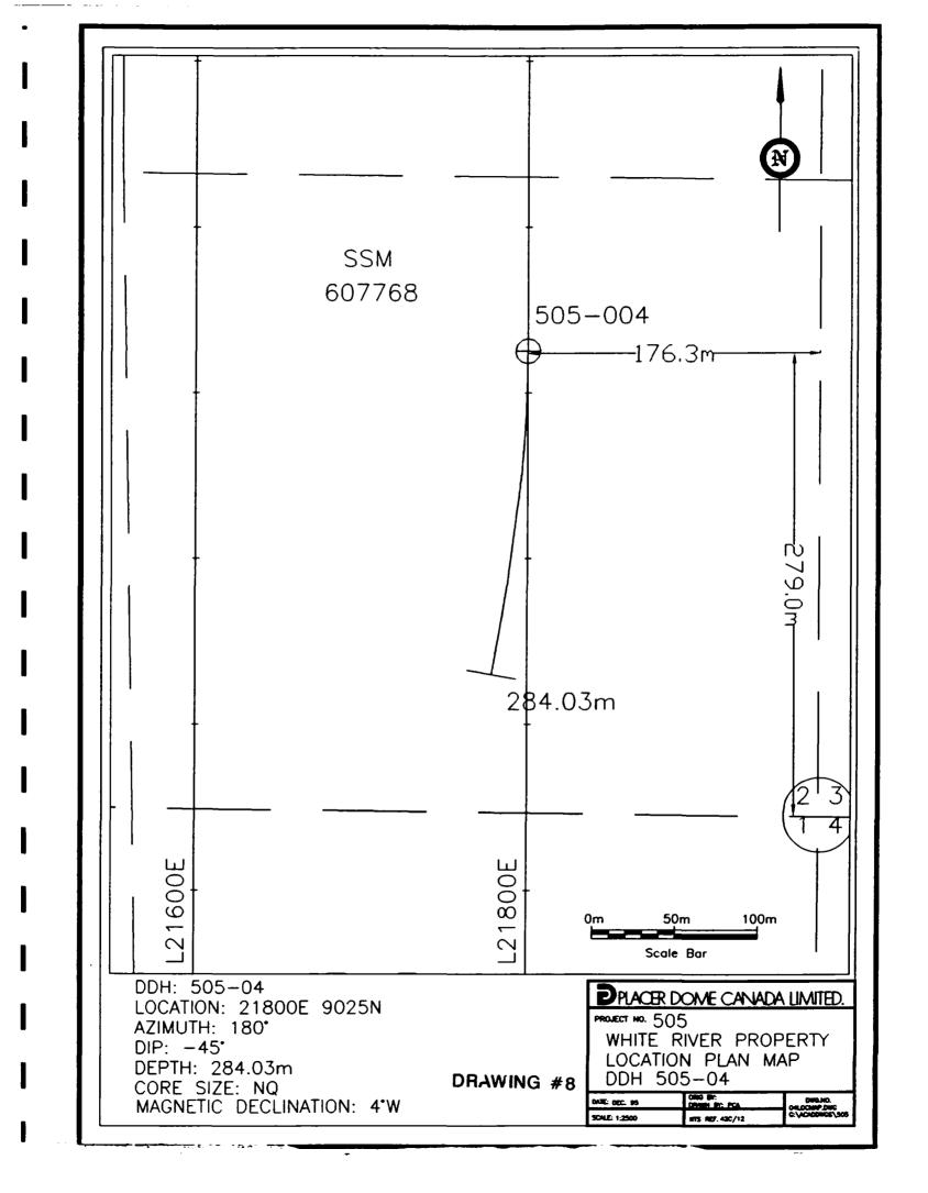
Date: 21st Dec, 1995 Northing 9025.00 Easting : Elevation : 21800.00 0.00 Hole Depth : 284.03mt Drill Hole Survey Data
