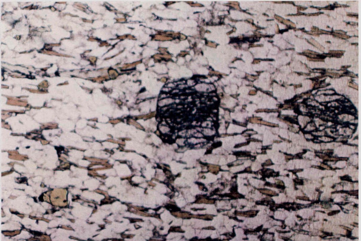
Sample 0505-013-276.00m: PP Light Photograph. Biotite Schist with Garnet Porphyroblasts. Note concordant fracture cleavage in garnets and disseminated yellowish coloured fine tourmaline
