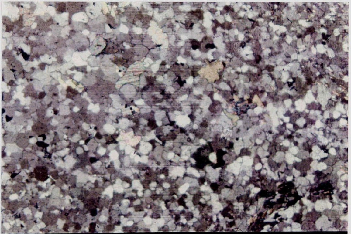
Sample 0505-008-210.99m: CP Light Photograph. Quartzo-feldspathic metasediment. Excellent granoblastic textures with quartz-plagioclase minor microcline, muscovite (light colours) and biotite. Very fine disseminated pyrite (black).
