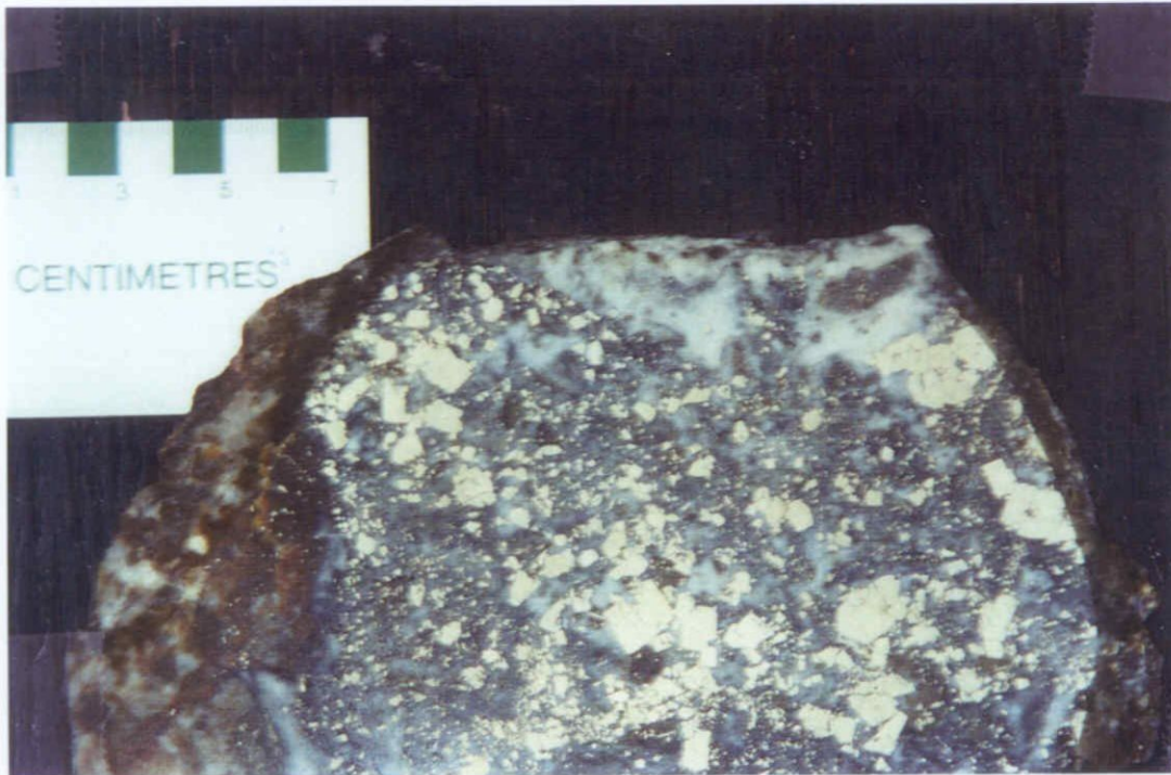
Photo 5: High Grade Au sample - Polished Slab – large pyrite cubes in quartz Matrix - fine wire gold within fractured pyrite cubes (sample assayed 25 oz Au per ton).
