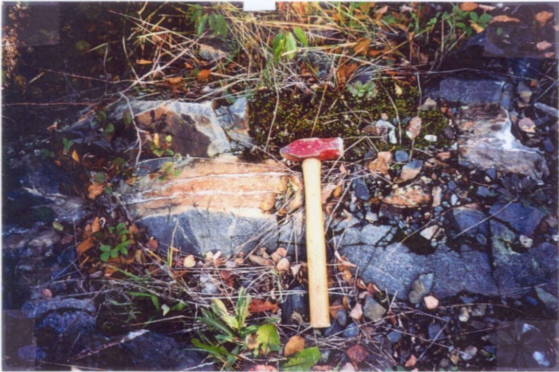
PHOTO #3: Very narrow quartz veins with brown pyritized, silicified alteration envelope. (Assayed 1191 ppb Au).
