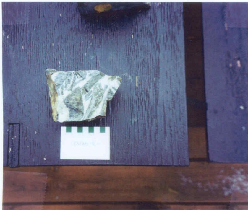
Photo 6: Quartz breccia vein – mafic angular metavolcanic clasts – assayed 7000 ppb Au.
