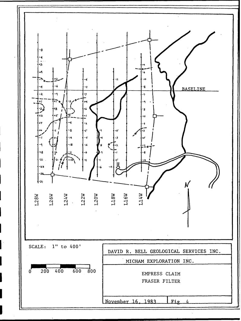
The conductor on line L14W at 4+50N cannot be readily explained but lies close to a presumed geological contact between the mafic flows and a gabbro.
