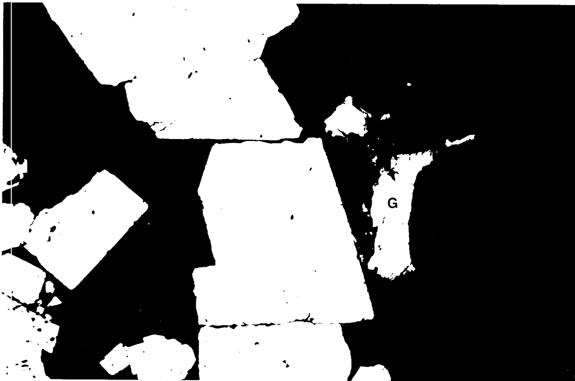
1328. Galena (g) with euhedral pyrite. Width of field: 4mm. Refl. light.
