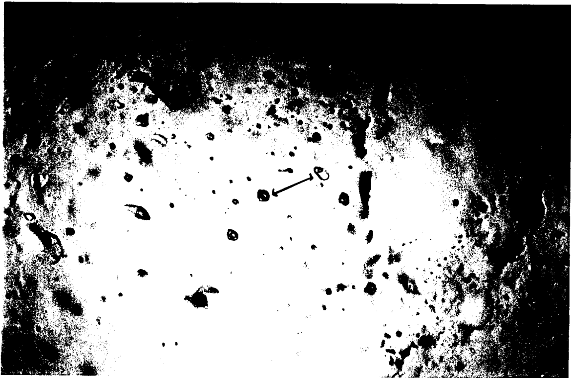
1465A. Possible evidence for boiling in fluid inclusions: large difference in vapor bubble sizes between 2 adjacent inclusions (arrow). Width of field: 0.45mm. Ppl.
