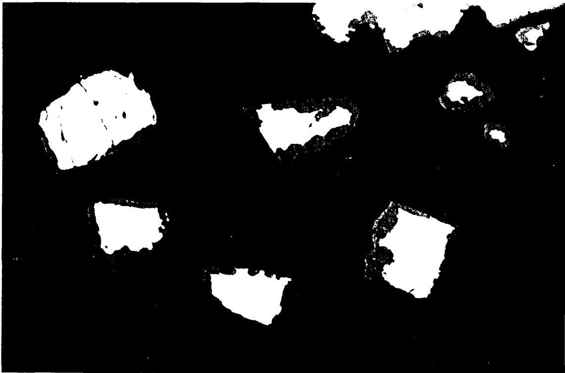
1465B. Pyrite grains are rimmed by hematite. Width of field: 4mm. Refl. light.
