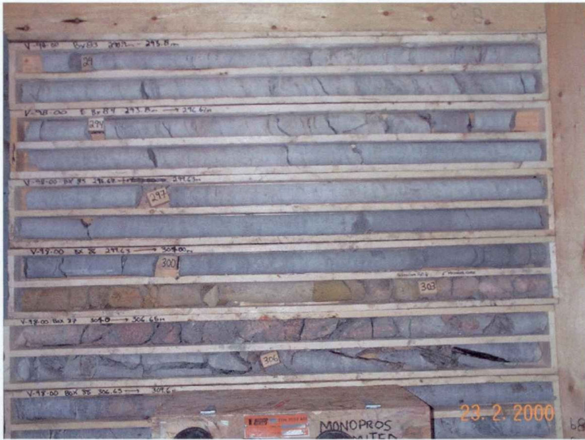
Figure 15: Upper two core boxes show the BCR dolostone and the fourth box shows the BCR basal sandstone.
