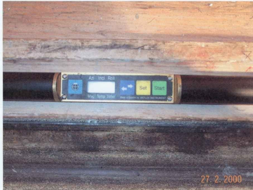
Figure 1 : Reflex down hole survey system
