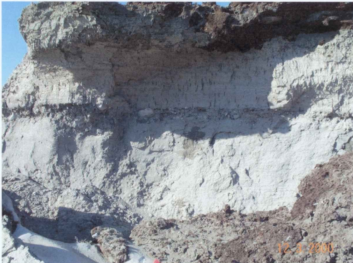
Figure 8: A 4m section of organics and overburden above Victor SW
