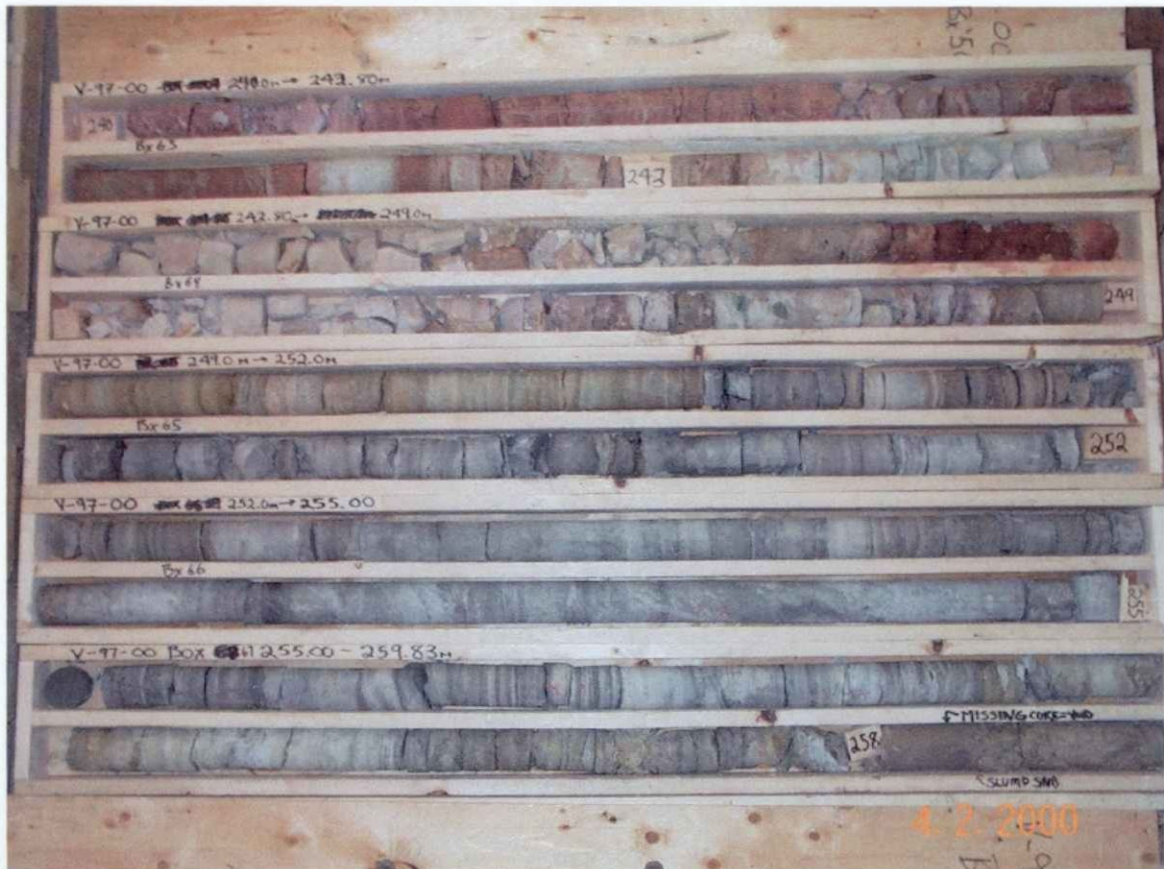
Figure 14: RH/CR Unit C Red Mudstone beds and finely bedded grey mudstone and evaporite sections. Very Weak Geotechnical units.
