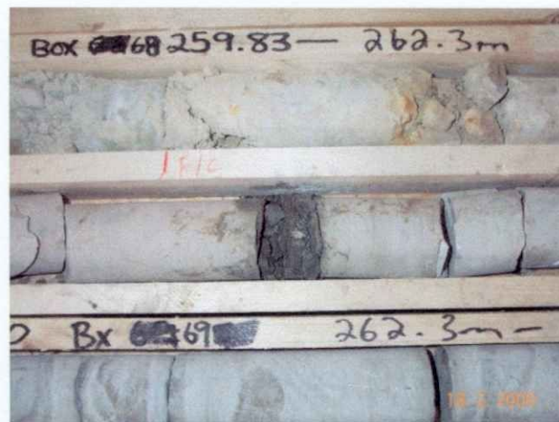
Figure 7 : 5-7 cm bed of petroliferous shale C Boas River Shale
