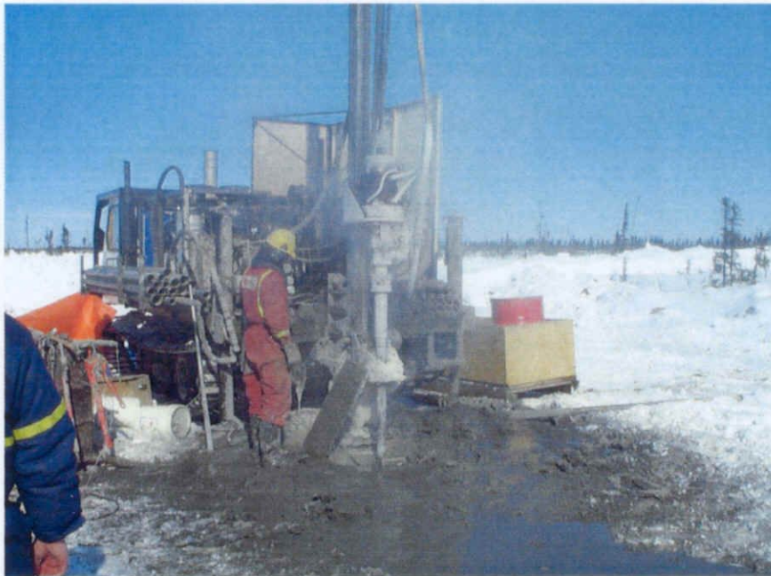
Figure 3. The RC-100 rig core-drilling with air.
