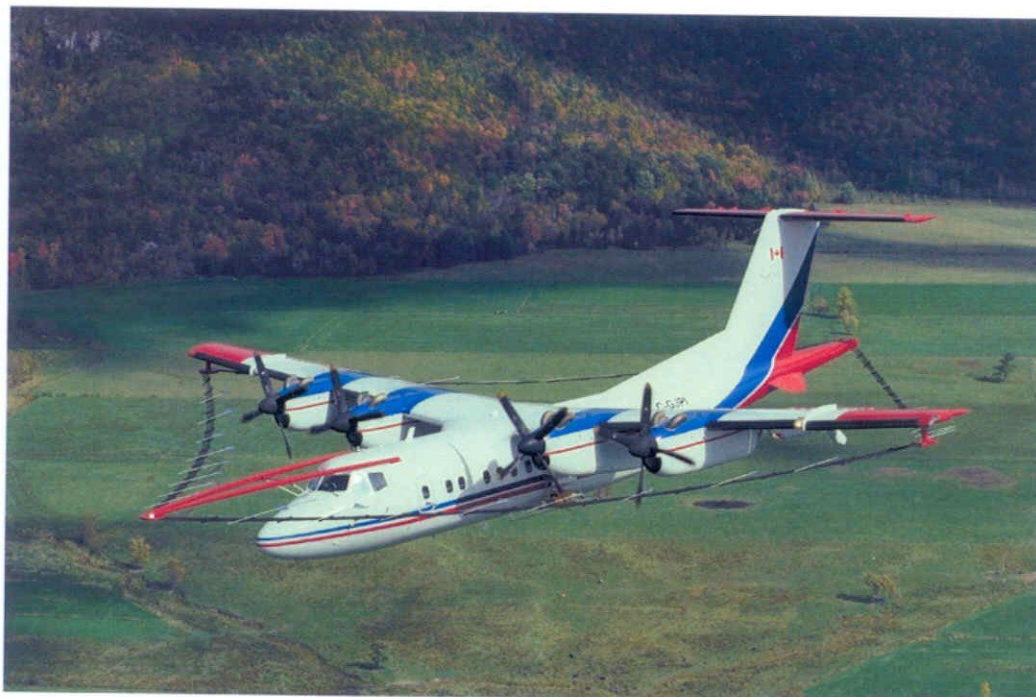
Figure 1: Specially modified Dash-7 aircraft used by Fugro Airborne Surveys.
