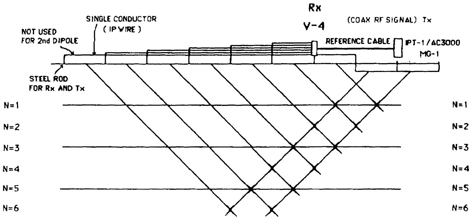
NOTE: V-4 CAN READ N-1 TO N-6 SIMULTANEOUSLY FROM TX DIPOLE
