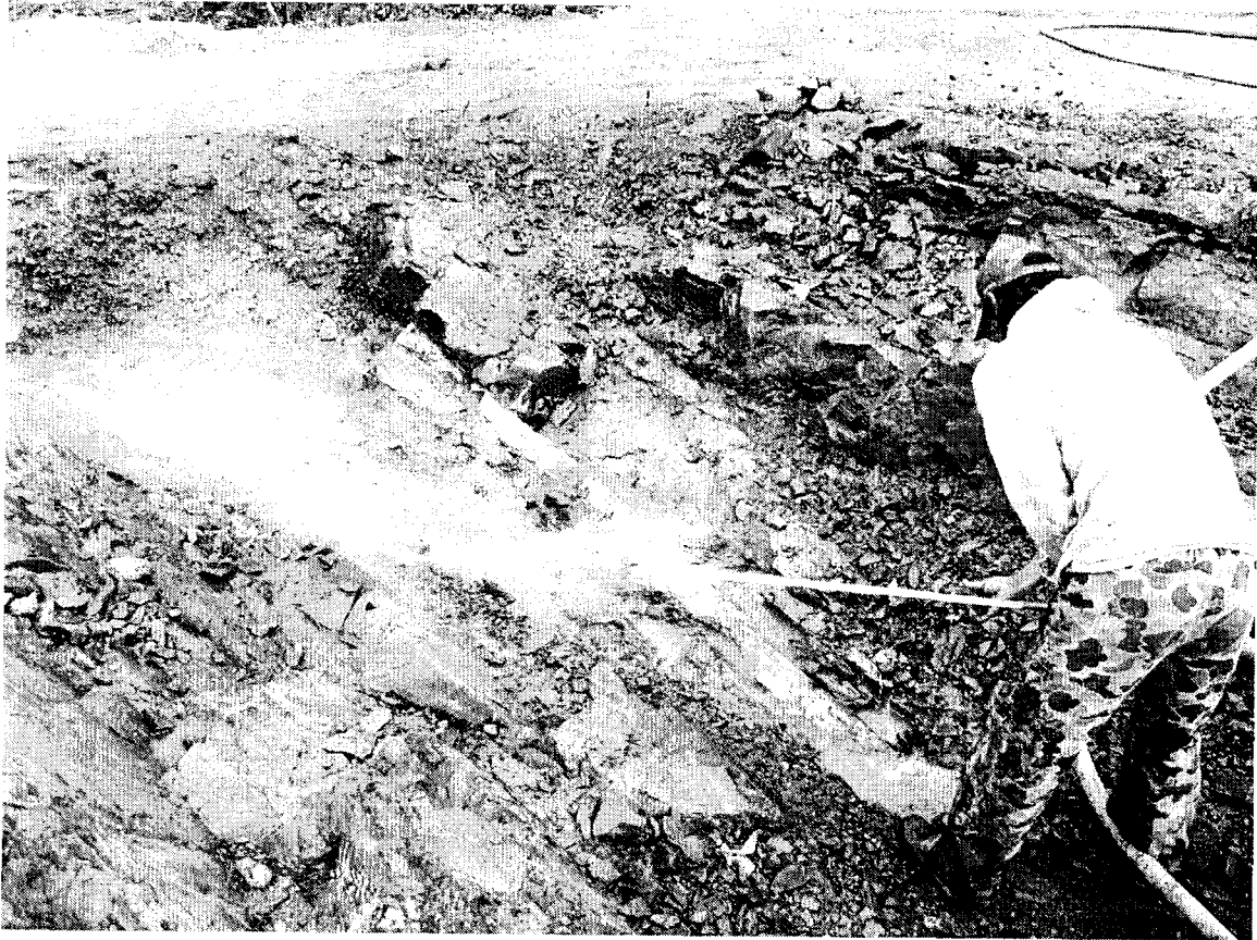
Power washing a quartz vein at the D65 showing.
