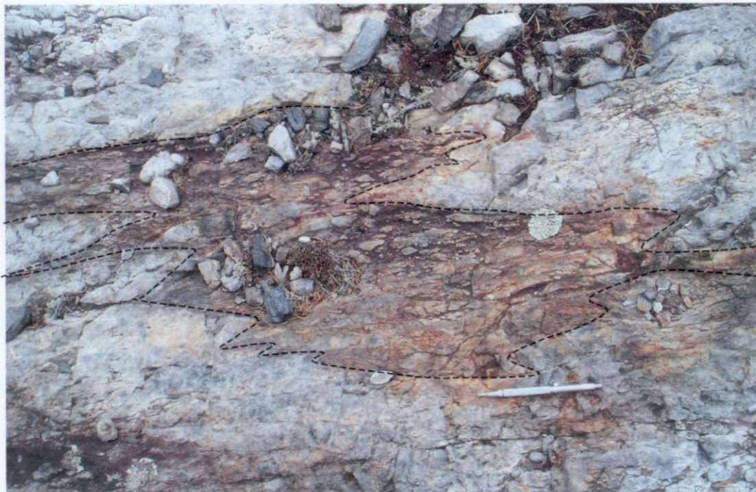
Figure 11 - Photograph showing transposed breccia zone with strong iron-oxide staining from main 991 outcrop.
