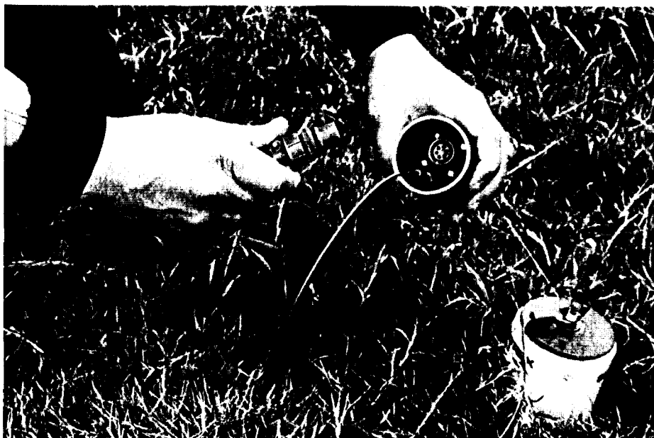
High production rates are obtained using Multidipole Potential Cables which permit measurement of six dipoles simultaneously.
