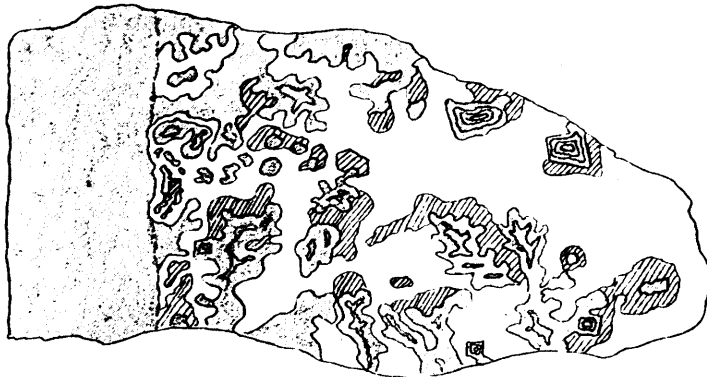
Fig. 30. Diagram of portion of vein from Silver Bar mine, natural size, showing order of deposition. The shaded part represents smaltite-chloanthite intergrowth with chloanthite in the centre of dendritic growths. The hatched part is later niccolite and the white is calcite.
