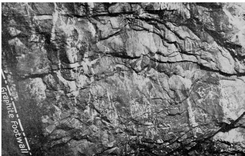
Ore body twenty-two feet wide on the 360-foot level, Associated Goldfields. The picture includes the ten feet next the footwall and shows white quartz cutting an altered, heavily mineralized, reddish tuff cut by quartz syenite.
