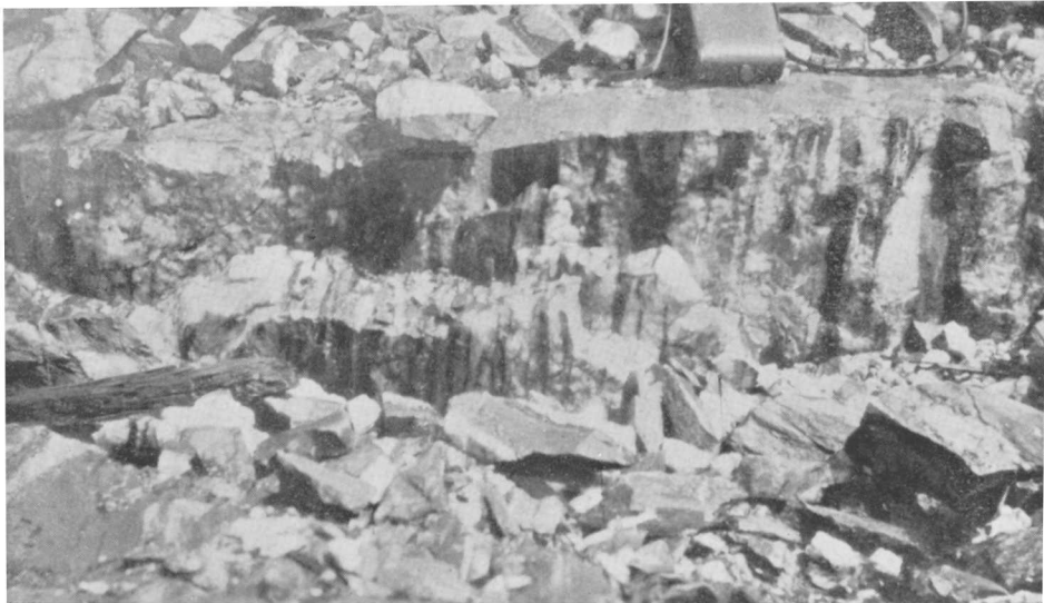
Ribbon type of quartz veins on the Howey ore body.
