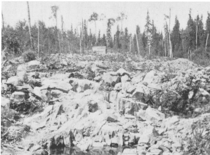
View of surface trenches on the Howey ore body looking west along the strike of the much fractured and sheared quartz porphyry.
