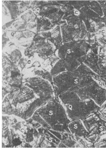
Fig. 1—Serpentine showing some calcite. (Crossed nicols \times 13 .) S=Serpentine. C=Carbonates. Q=Quartz.
