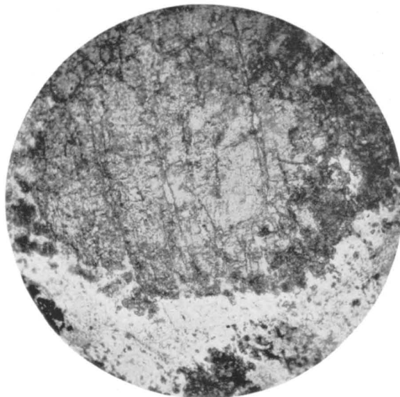
Photomicrograph of gabbro-porphyrite showing the alteration of a phenocryst to saussurite (dark) and the serpentine-chlorite matrix (light). ( \times 30 .)
