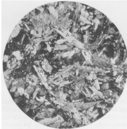
Photomicrograph of andesite porphyry (groundmass only, phenocrysts not shown). The groundmass is a felt of andesine (A) and hornblende laths with dark interstitial material ( \times 31 ).
