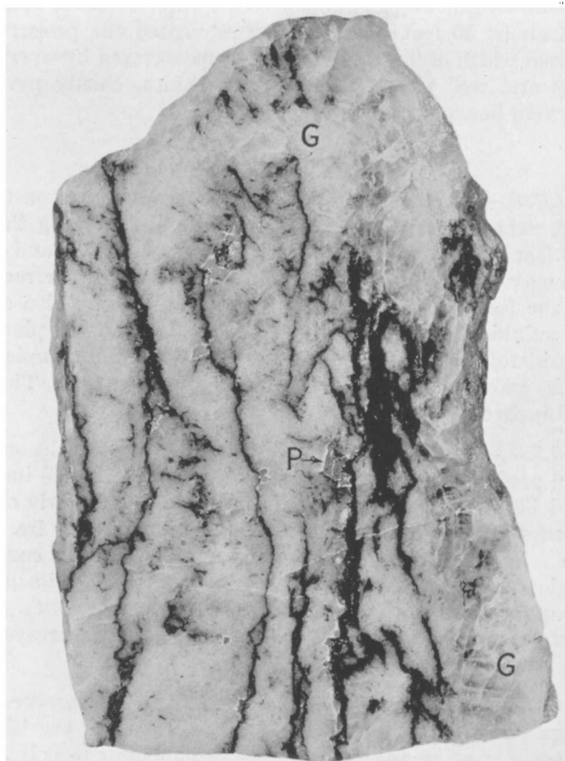
Polished sample (natural size) of gold ore from No. 3 vein, Kenricia Gold Mines. Sugary quartz with black tourmaline and pyrite (P) is cut by a slightly later generation of glassy white quartz (G).
