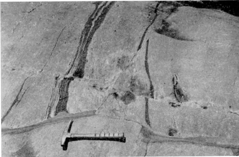
Detail of complex minor block faulting in anorthosite containing narrow bands of hornblende rock, west shore of Parry island, half a mile north of Caswell bay. The marks on the hammer handle are 1 inch apart.
