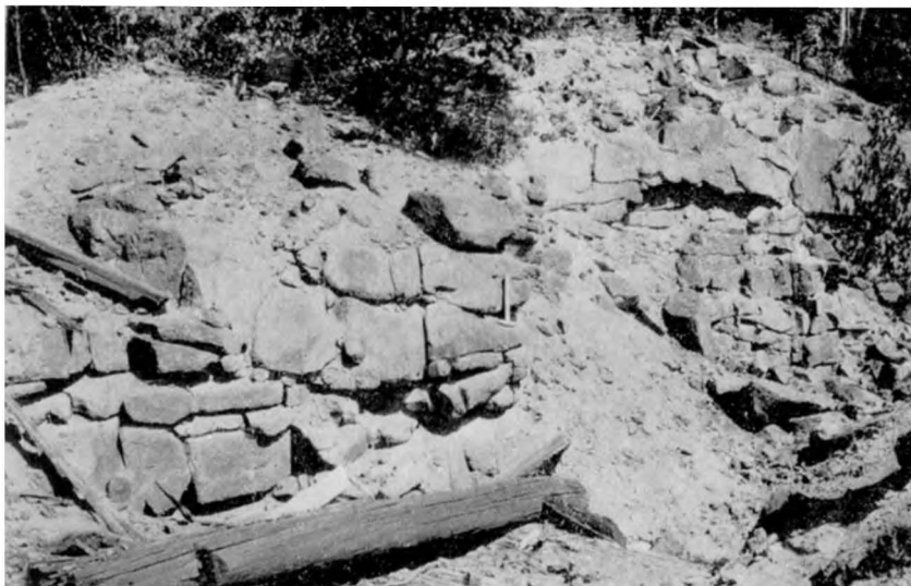
Spheroidal weathering of well-jointed norite, open cut and old shaft (covered in the foreground), Kelcey showing, Memesagamesing lake, lot 23, concession VIII, Hardy township.
