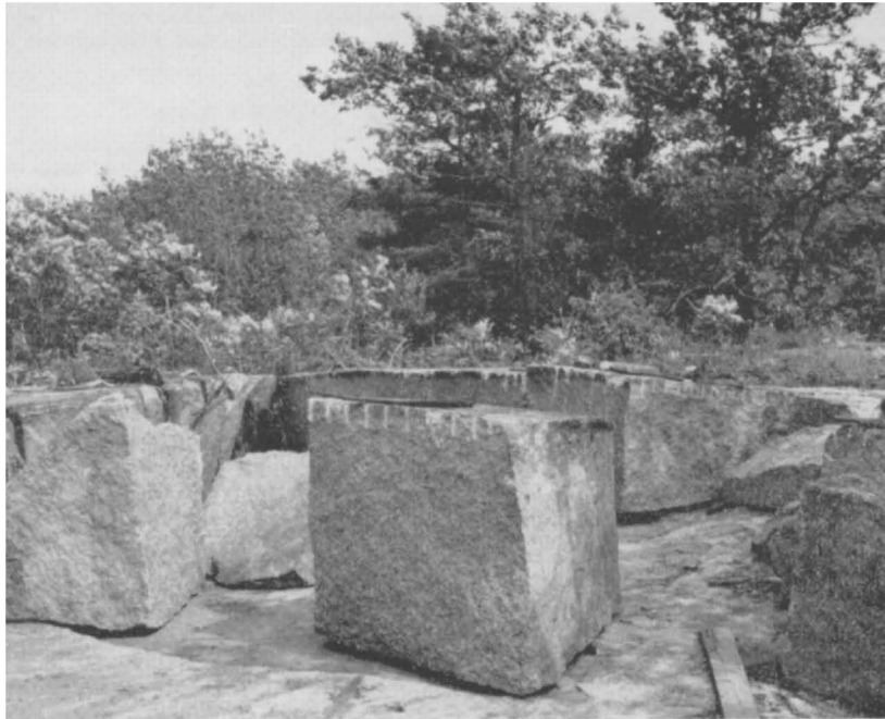
Mill block, 3 by 4 by 5 feet, of porphyritic biotite granite in the quarry of the Stoney Lake Granite Quarries, Limited, on lot 32, concession XII, Dummer township, Peterborough county.
