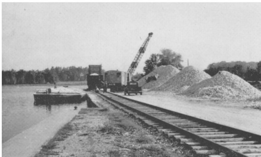
Austin clam at dock, Lakefield, unloading nepheline syenite from scows, June, 1942. A 20,000-ton stock pile is built up each year at this dock for transhipment by rail to Cobourg and rail ferry to the mill of the American Nepheline Corporation at Rochester.
