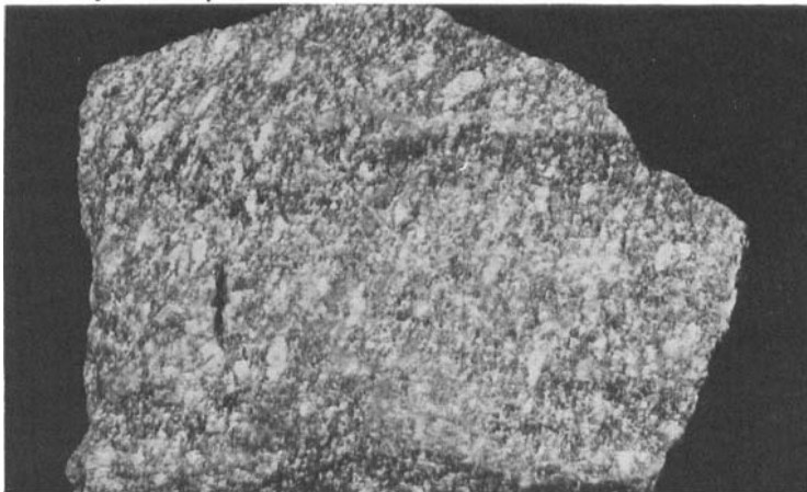
Photo 18 Sample of porphyritic syenite from quarry west of the Rainy Lake Causeway. The sample is 8 inches across.
