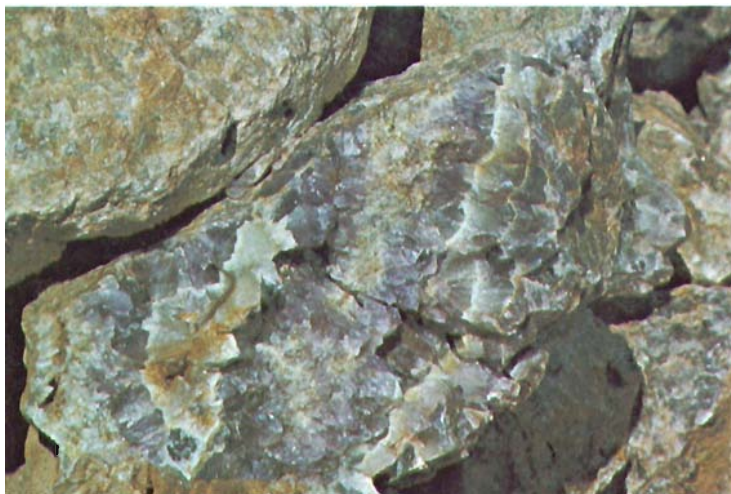
Photo7. Zoning of amethyst and quartz in mineralized breccia of the Thunder Bay Amethyst Mine indicates changing conditions in the mineralization process. (Courtesy Ont. Min. Industry and Tourism).
