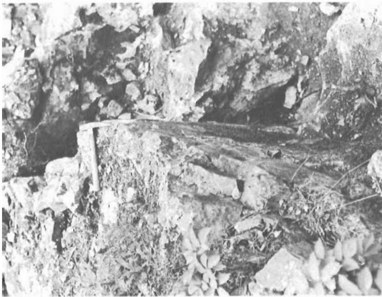
Photo 24. In the excavation on Druba's property (see photo 23) semi-cylindrical blocks of quartz monzonite are exposed. The blocks have curved slickensides as indicated by the hammer head. Movement took place in a near vertical direction.
