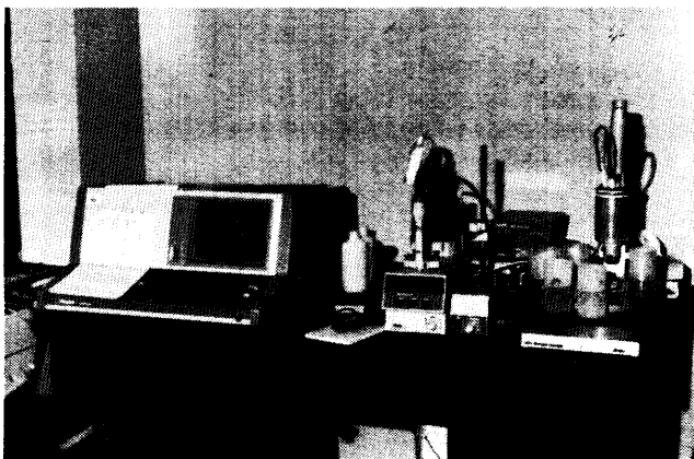
Photo 33.1. Metrohm AG titroprocessor as configured at the Geoscience Laboratories Toronto facility. Titroprocessor (left), dosimat (central) and sample changer (right), keyboard of LIMS computer just seen on far left.
