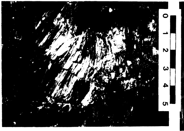
Photo 7.4. Coarse, white to pale green tremolite aggregates associated with massive white dolomite and white to pale green diopside on the southwest shore of Palmerston Lake (UTM 18T 352720E 4985400N).
