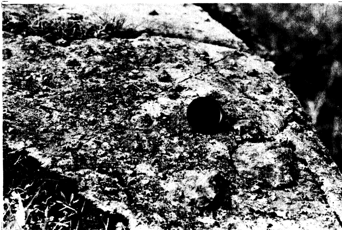
Photo 20: High-relief weathering of quartz knots in impure dolomitic marble (ROSS-03).
