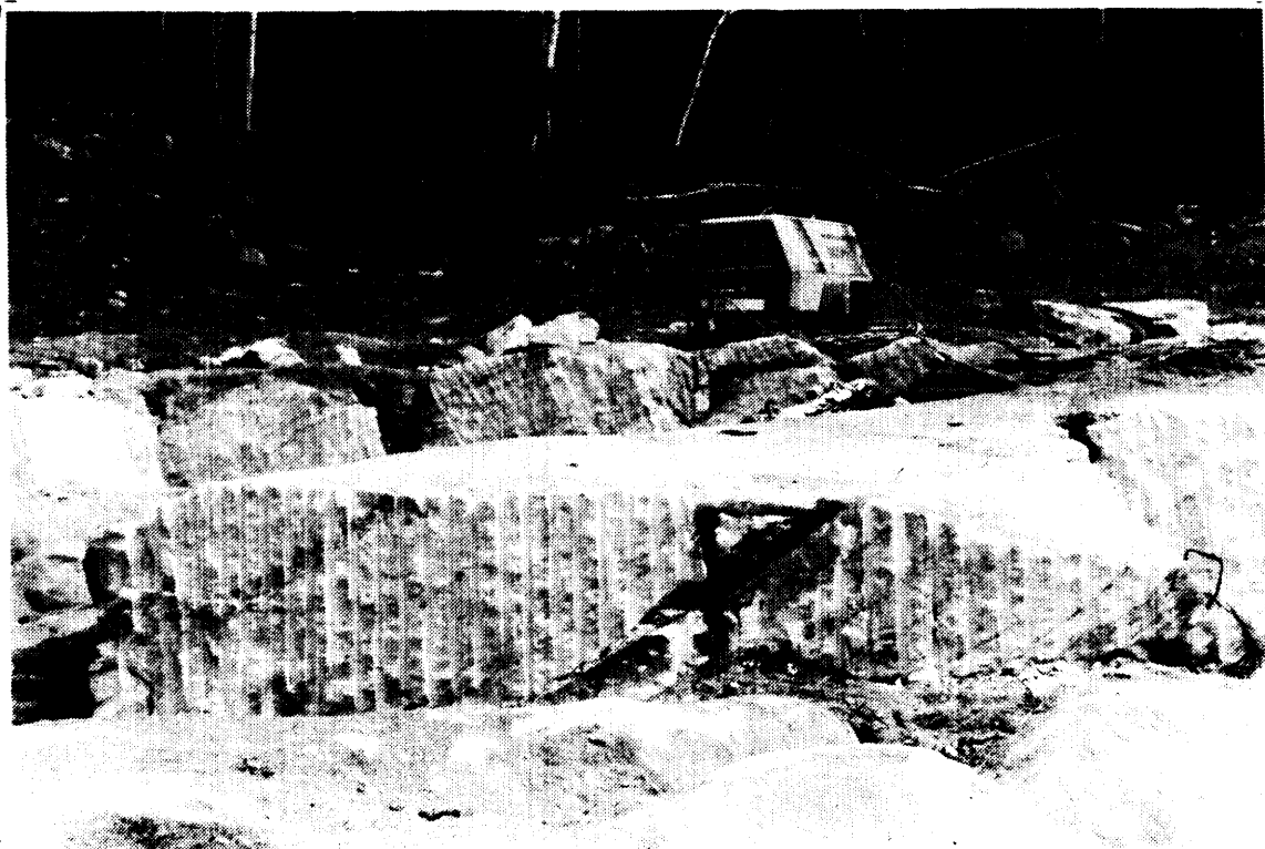
Photo 9: Dimension stone quarry (GRI-02), May 1989, showing white, calcitic/dolomitic marble with pale green, serpentine-rich bands.
