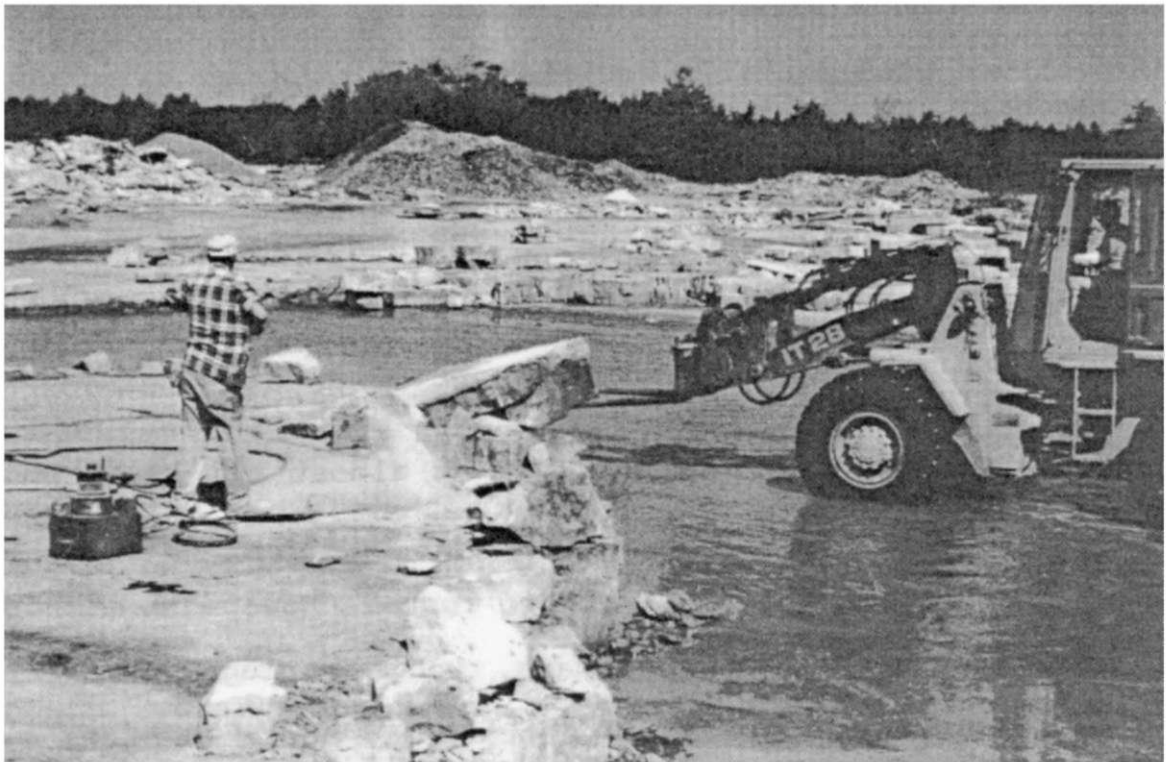
Photo 3. Quarrying a 55 cm thick dolostone bed using a pneumatic rock drill and forklift, Owen Sound Ledgerock, Wiarton quarry.
