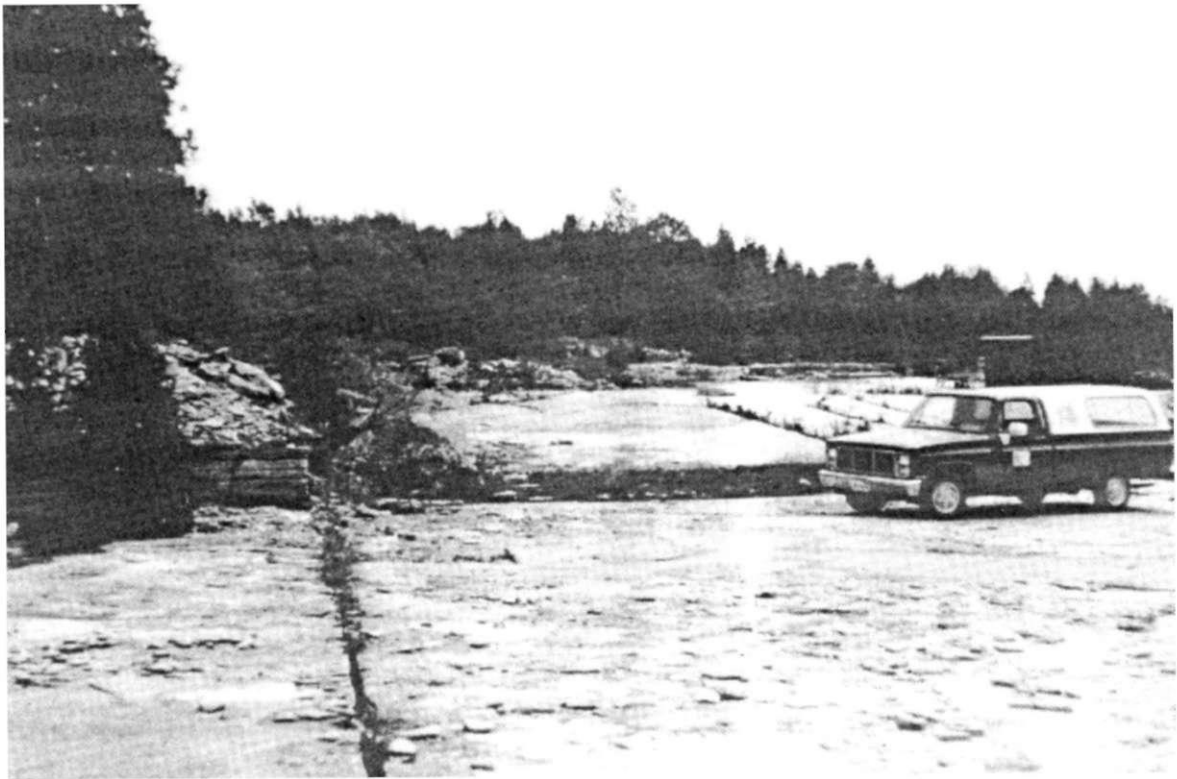
Photo 7. Limestone pavement showing widely spaced joints, J.S. Cook quarry, Wiarton.
