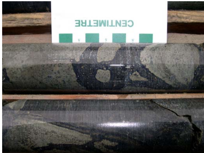
Photo 18. Brecciation at the base of the lower intrusion from Falconbridge drill hole G32-25 (04-SMH-0001).
