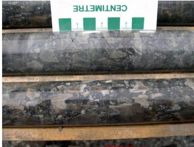
Photo 6. Felsic hyaloclastite from Falconbridge drill hole G32-25 (04-SMH-0001).
