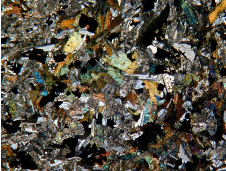
Photo 54. Photomicrograph of coarse-grained Matachewan diabase intrusion in crossed polarized light. Sample 03-SMH-0022. Field of view is approximately 22 mm.
