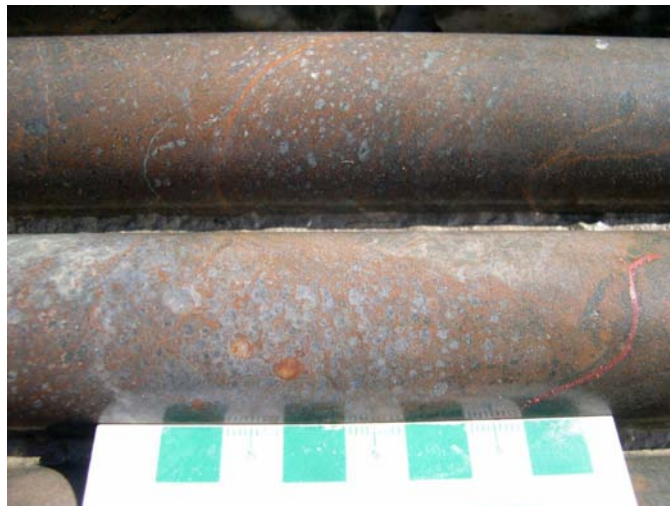
Photo 42. Massive Fe-carbonate alteration in mafic intrusion from Falconbridge drill hole G22-15 (04-SMH-0003).
