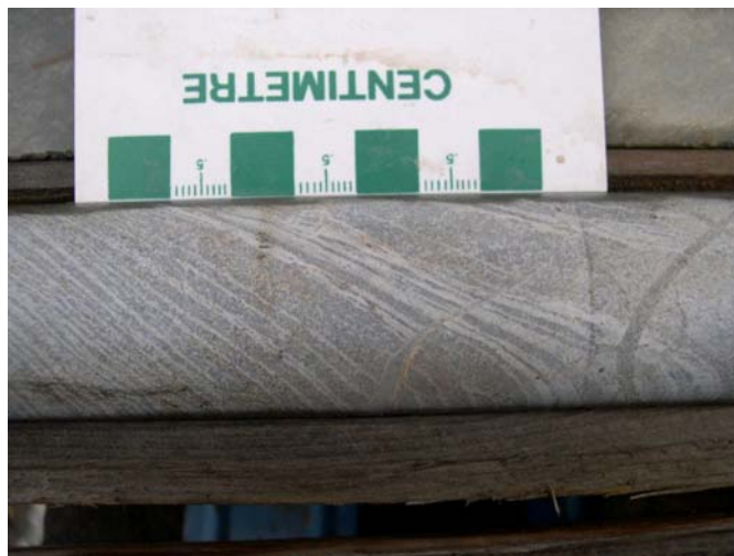
Photo 26. Bedded-tuff from Falconbridge drill hole G22-12 (04-SMH-0005).
