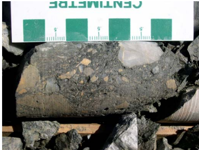
Photo 25. Heterolithic lapilli-tuff breccia from Falconbridge drill hole G32-10 (04-SMH-0024).
