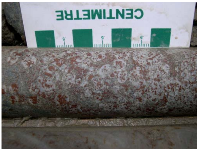
Photo 5. Spherulites in felsic flow from Falconbridge drill hole G22-12 (04-SMH-0005).
