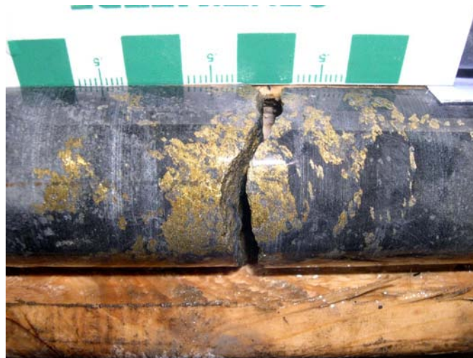
Photo 46. A-zone sulphide mineralization in intermediate synvolcanic intrusions from Explorers Alliance drill hole EGG32-35 (04-SMH-0007).
