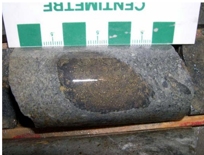
Photo 28. Mineralized mudstone fragment in lapilli-tuff from Falconbridge drill hole G22-12 (04-SMH-0005).
