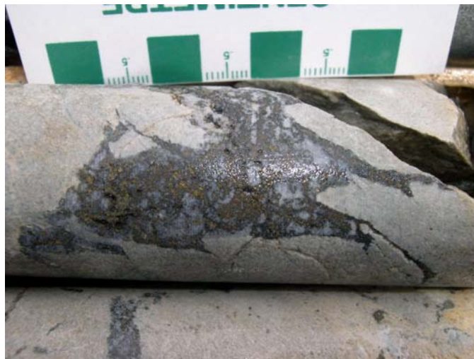
Photo 48. Black sphalerite mineralization in “Claim Post zone” from Explorers Alliance drill hole EGG32-32A (04-SMH-0013).
