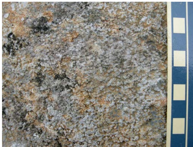
Photo 39. Outcrop appearance of Fe-carbonate alteration in massive mafic unit (03-SMH-0127).
