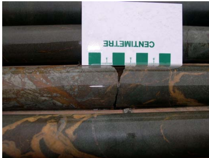
Photo 41. Fe-carbonate veins in mafic unit from Falconbridge drill hole G22-14 (04-SMH-0002).
