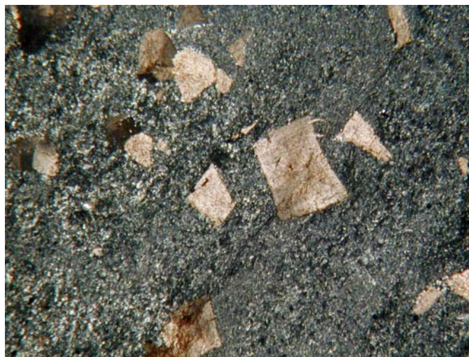
Photo 40. Photomicrograph of Fe-carbonate rhombs (03-SMH-0073: field of view is approximately 22 mm).
