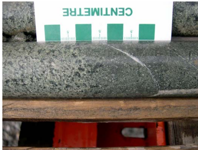
Photo 16. Coarse- to medium-grained intrusion from Falconbridge drill hole G32-26 (04-SMH-0023).
