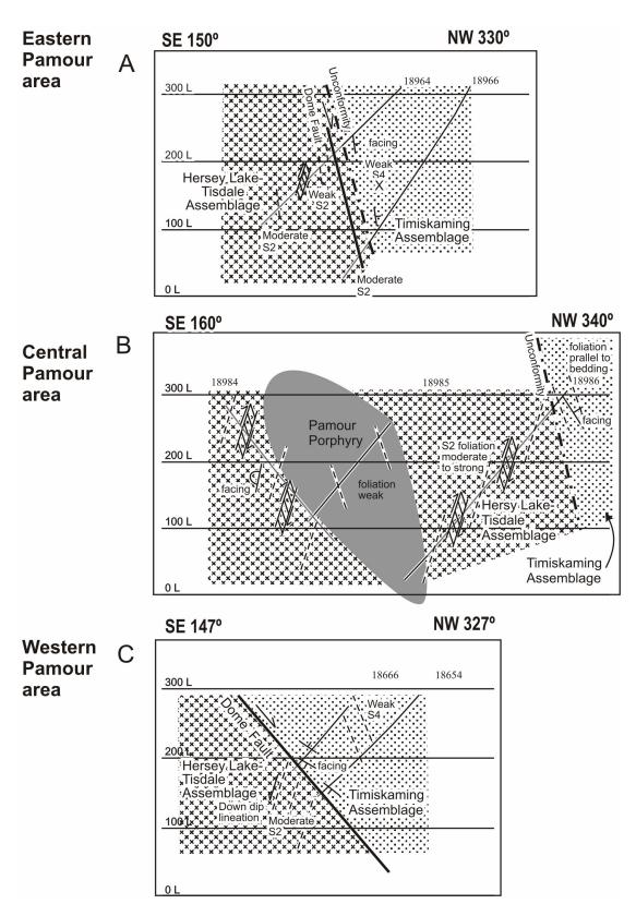
**Figure 24.** Three cross-sections through the Porcupine–Destor deformation zone, as mapped in diamond drill holes. Location of section shown in Figure 3.
