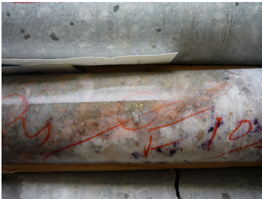
Figure 4. Gold-bearing, altered granodiorite with visible gold and fluorite in quartz vein, Dingman property, Upper Canada Gold Corporation. Core diameter is 4.75 mm. Photo by J. Chard.
