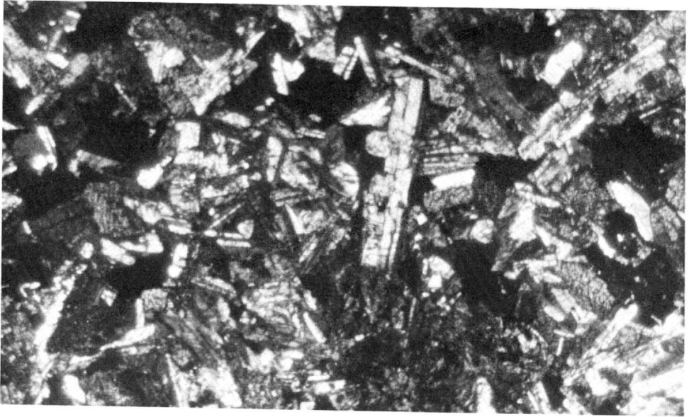
Photo 9—Photomicrograph (40X) of medium-grained diabase, showing doleritic texture. Approximately 0.5 km southeast of Perrault Lake.
