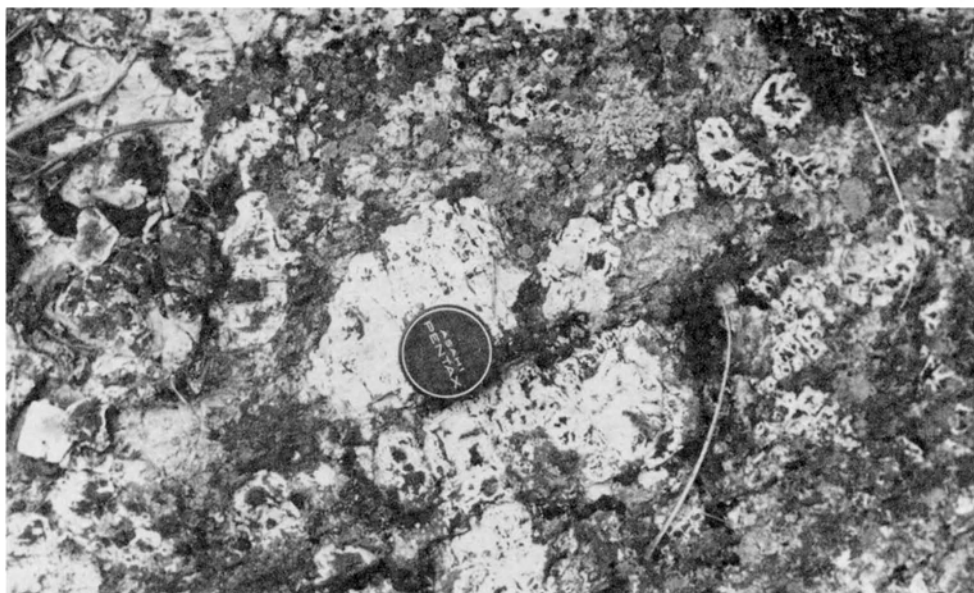
Photo 7—Nepheline syenite pegmatite from the South Algona-Sebastopol Townships nepheline syenite zone. The nepheline is creamy white with black stains, the albite is grey.
