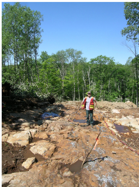
Photo 19. Site 5c. The main trench at Trill showing the rusty central core of mineralized inclusion quartz diorite (IQD) flanked on both sides by barren quartz diorite (QD).
