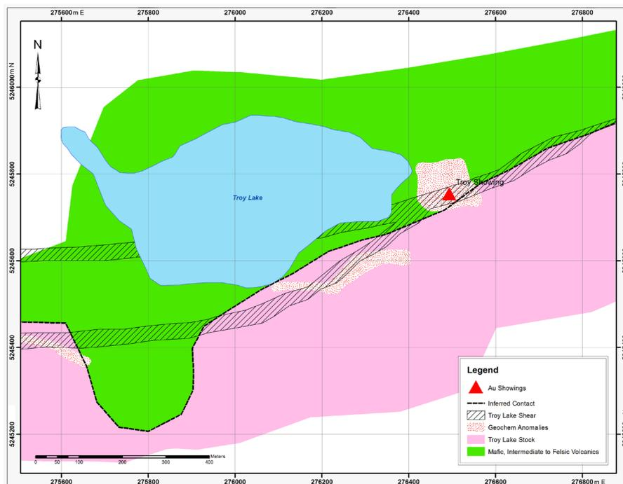
**Figure 2.** Map of the immediate area surrounding Troy Lake, showing the location of the Troy Lake gold showing (red diamond) and east-west-trending Troy Lake shear zone, as well as the 3 gold anomalies in overburden occurring along the Troy Lake shear zone. (From Perk 2009).
