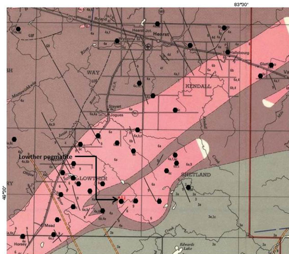
**Figure 1.** Location of Lowther pegmatite in Lowther Township. The black hexagons represent areas where pegmatitic rocks were recorded by the OGS. Modified from OGS Map 2166 (Bennett et al. 1969).
