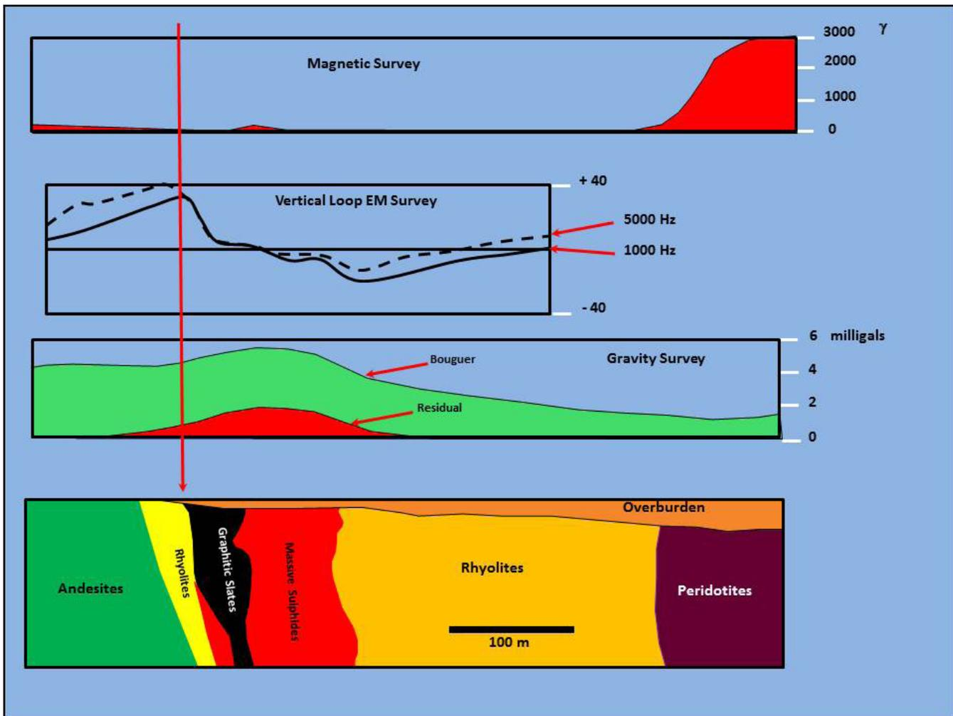
**Figure 3.** Geophysical response over the Kidd Creek VMS deposit (after Donohoo, Podolsky and Clayton 1970; and Bleeker 1999).
