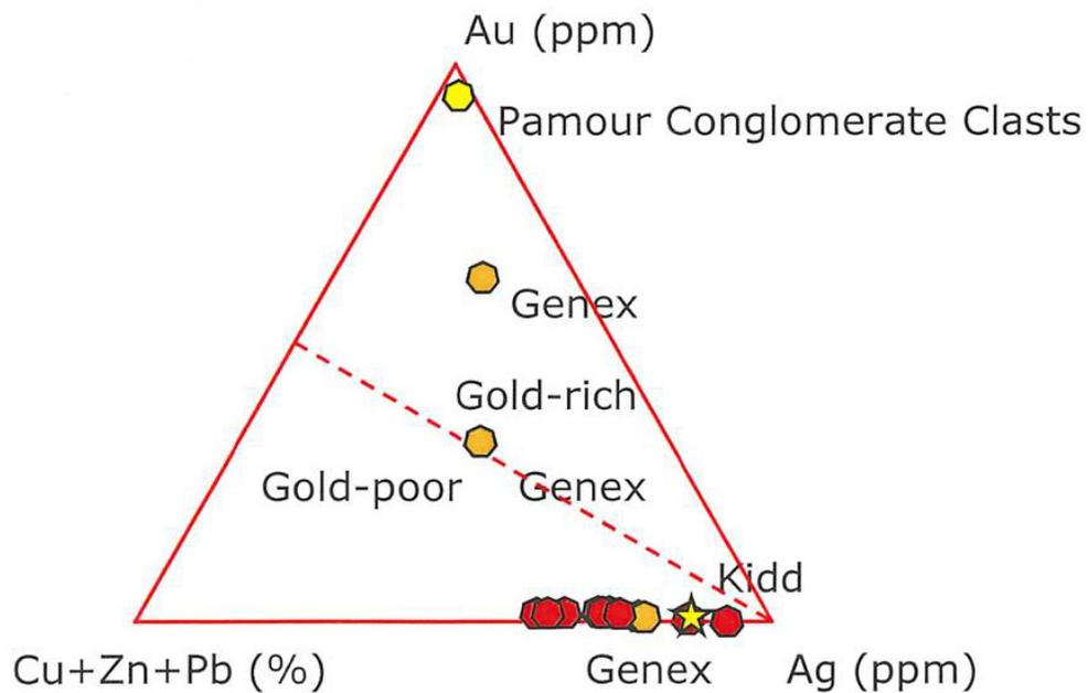
**Figure 1.** Ternary plot of Cu+Zn+Pb, Ag and Au content in Porcupine area VMS deposits or prospects. Red hexagons indicate the Canadian Jameson, Jameland, Kam Kotia and Potter deposits and Chance, Halfmoon, Terminus and Tillex prospects. The Kidd Creek deposit is indicated by a yellow star, Genex deposit by orange hexagons and pyrite clasts in Pamour conglomerate by a yellow hexagon. (After Galley et al. 2005.)
