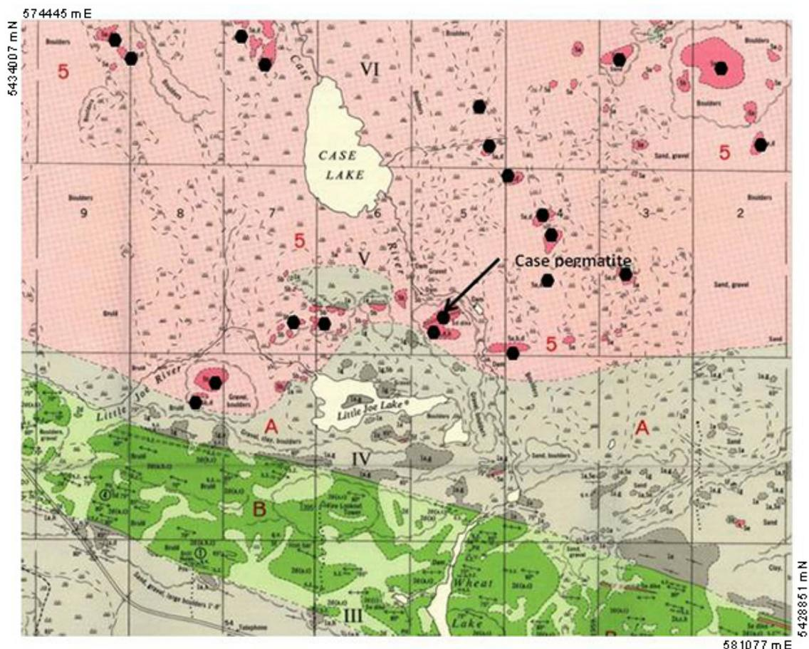
**Figure 2.** Case pegmatite. The black hexagons represent areas where pegmatitic rocks were recorded by the OGS. *Modified from OGS Map 2018 (Lumbers 1962).* Universal Transverse Mercator (UTM) co-ordinates, in North American Datum 1927 (NAD27), Zone 17, are approximate.
