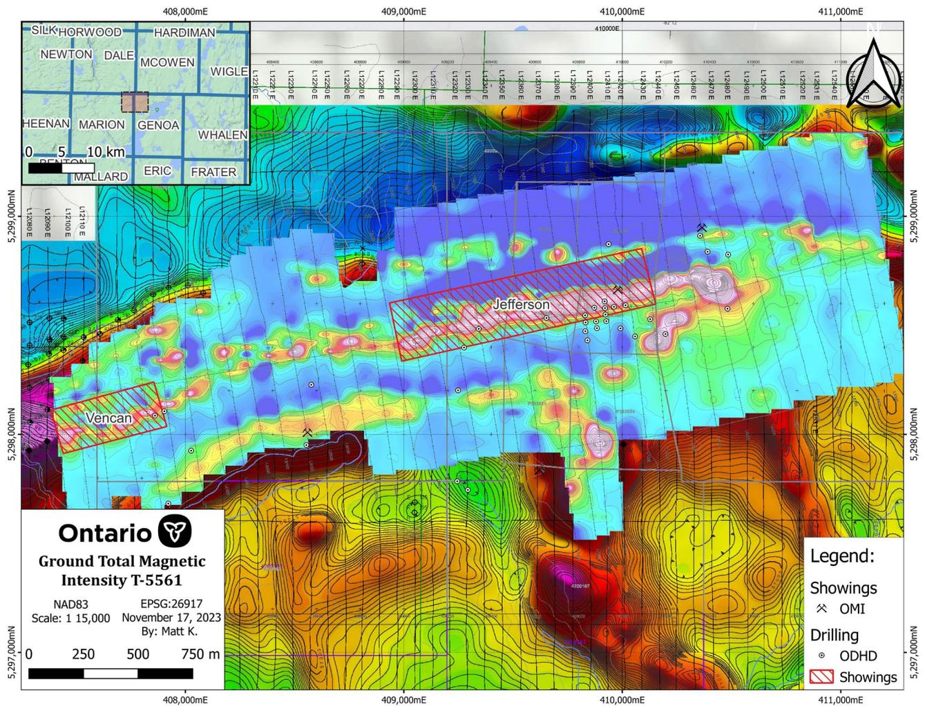
**Figure 4.** Ground based total magnetic intensity survey from assessment file T-5561 (Grant 2006), illustrating more detailed resolution than the manned airborne survey shown in Figure 3.
