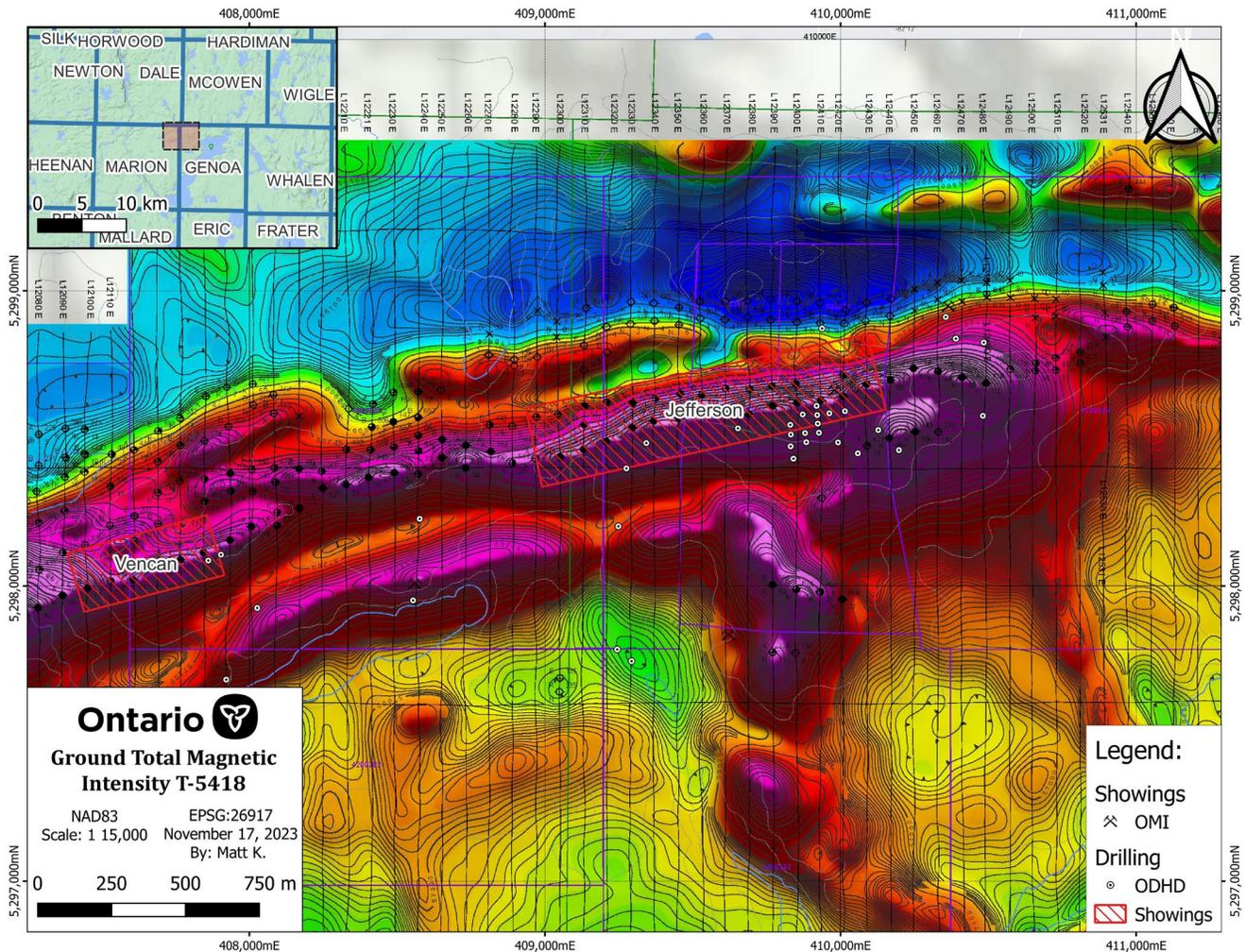
Figure 3. Airborne total magnetic intensity survey from assessment file T-5418 (Simon et al. 2006).
