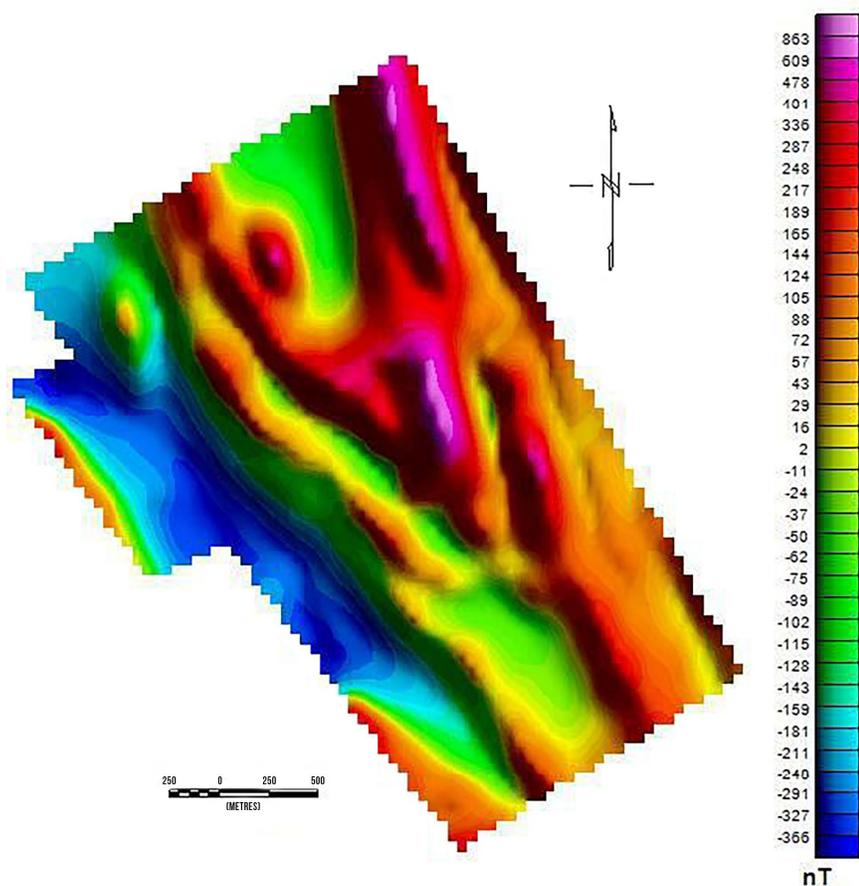
**Figure 1.** Helicopter-borne magnetic geophysical survey map. Total residual magnetic field data (M. Burns, CEO Pioneer Exploration Consultants Ltd., personal communication, 2023).
