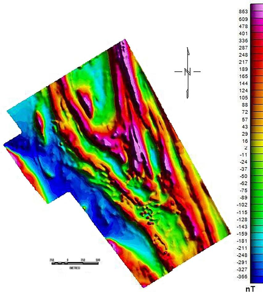
**Figure 2.** Drone-based magnetic survey map for same area shown in Figure 1. Residual total magnetic field data. Note the greater resolution compared with Figure 1 (M. Burns, CEO Pioneer Exploration Consultants Ltd., personal communication, 2023).
