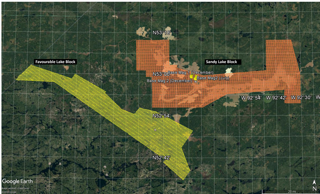
Figure 2. Flight path and magnetic base station locations displayed on Google Earth™ image.
