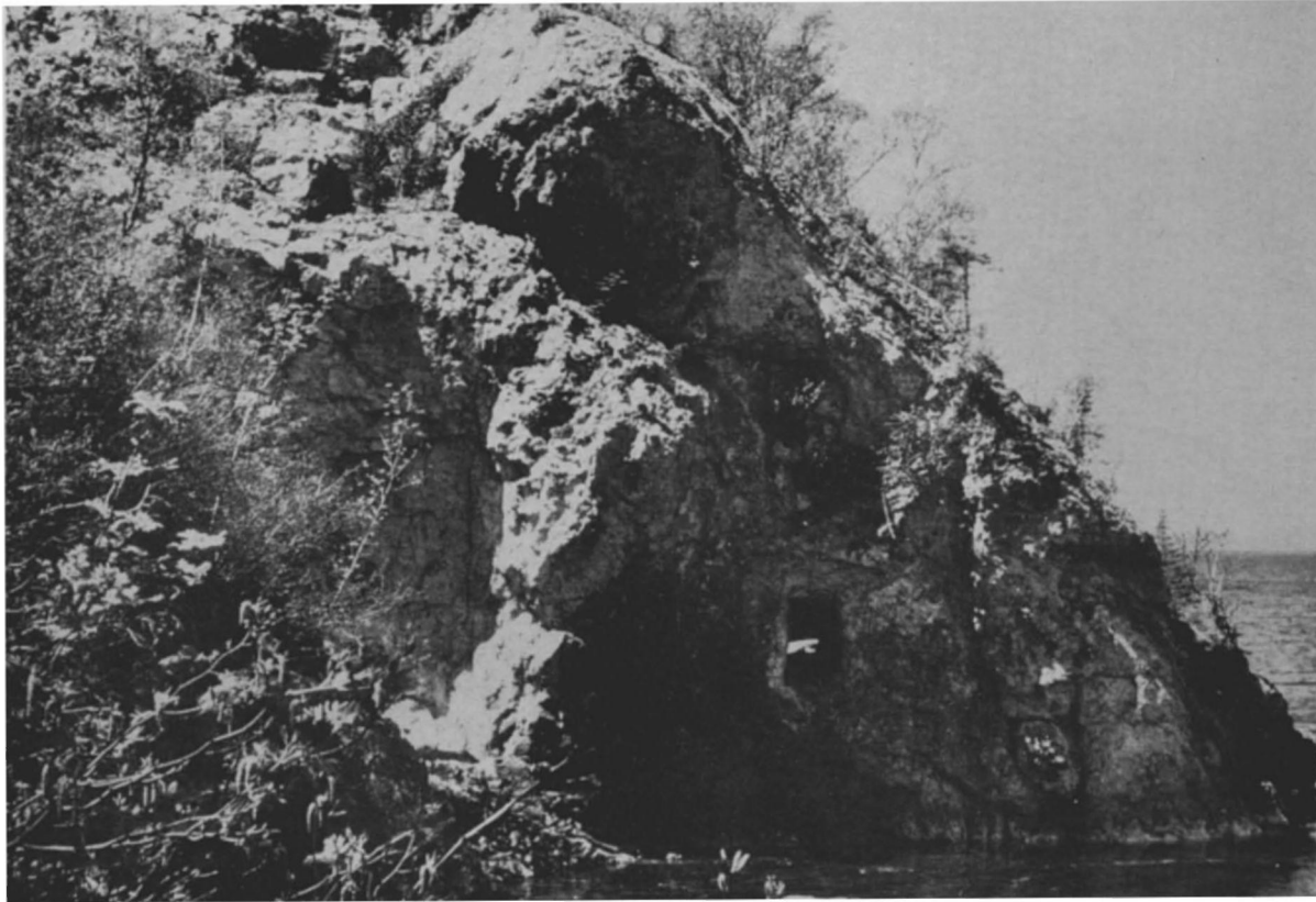
McKellar Island, north side, showing the adit entrance in the steep northeast flank of the barite vein. The adit crosses the width of the vein and connects with a narrow open-cut paralleling the west contact. The adit opening is 4 feet by 6 feet, and is about 8 feet above water-level.
