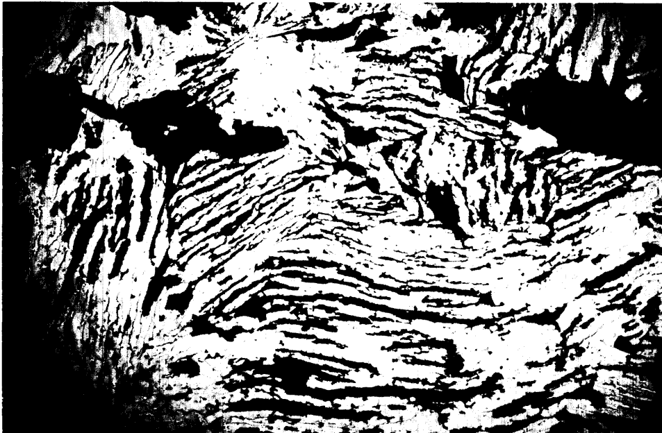
Photo 21—Photomicrograph showing a skeletal eutectoid-like intergrowth of chalcopyrite (light gray), marcasite (white) and gangue material (dark gray). Plane polarized light. Photo by W. Hicks, Ontario Division of Mines.
