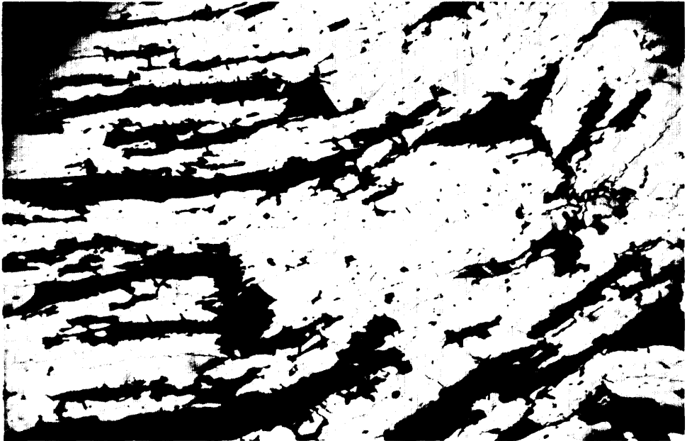
Photo 22—Photomicrograph showing fine detail of the chalcopyrite-marcasite intergrowth seen in Photo 21 (plane polarized light). Photo by W. Hicks, Ontario Division of Mines.
