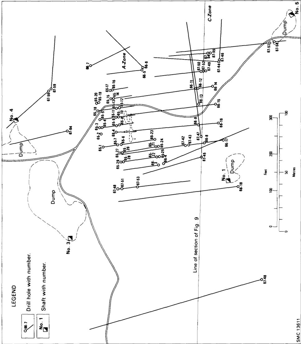
Figure 8—Plan of shafts of Mann Mine (26) and diamond drilling on the "A", "B", and "C" zones. Modified from plans of Manridge Mines Limited.
