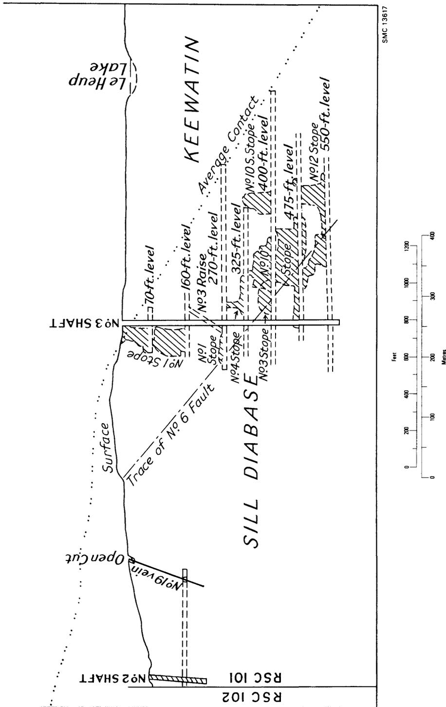
Figure 14—Longitudinal section through shafts No. 2 and No. 3, Castle Trethewey Mine (73). (Burrows 1926, p. 35).
