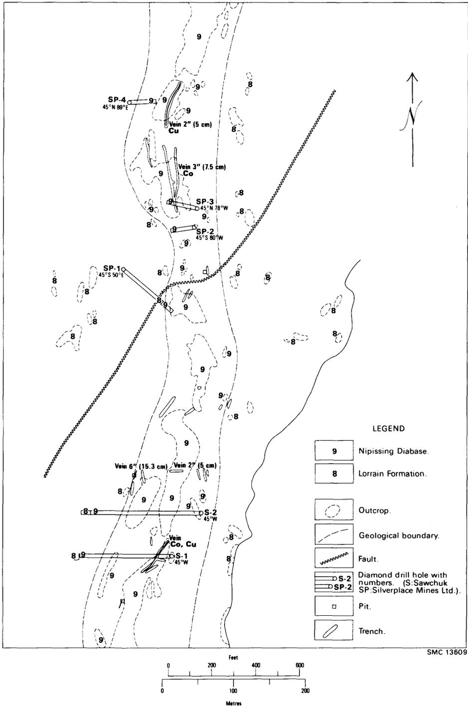
Figure 6—Plan of diamond drill holes, trenches, and veins on Silverplace Mines Limited [1965] (4). Modified from assessment work data.
