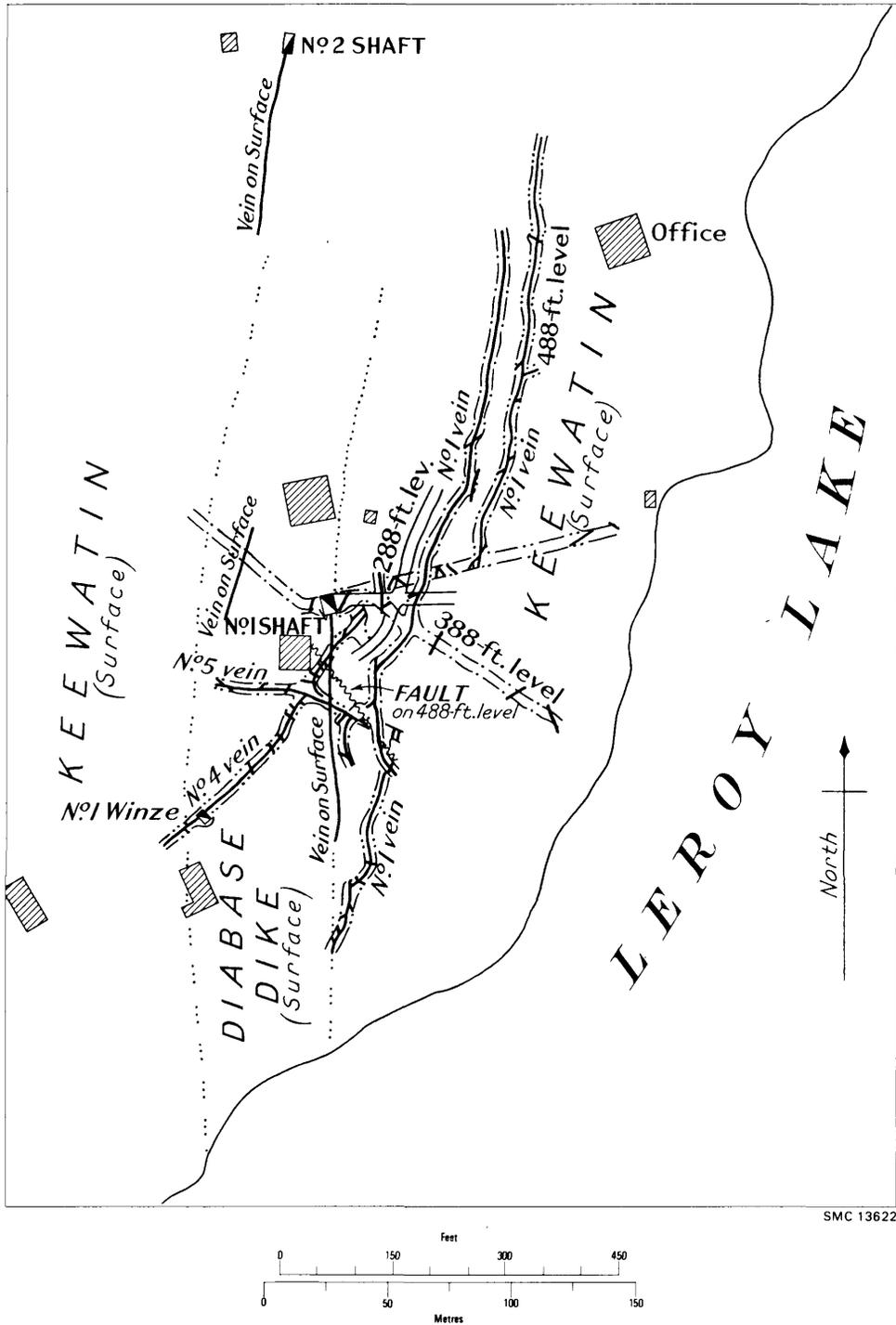
Figure 19—Underground plans at the Coleroy Gowganda Mine (116) held in 1969 by Silver Bar Mines Limited (Burrows 1926, p.45).
