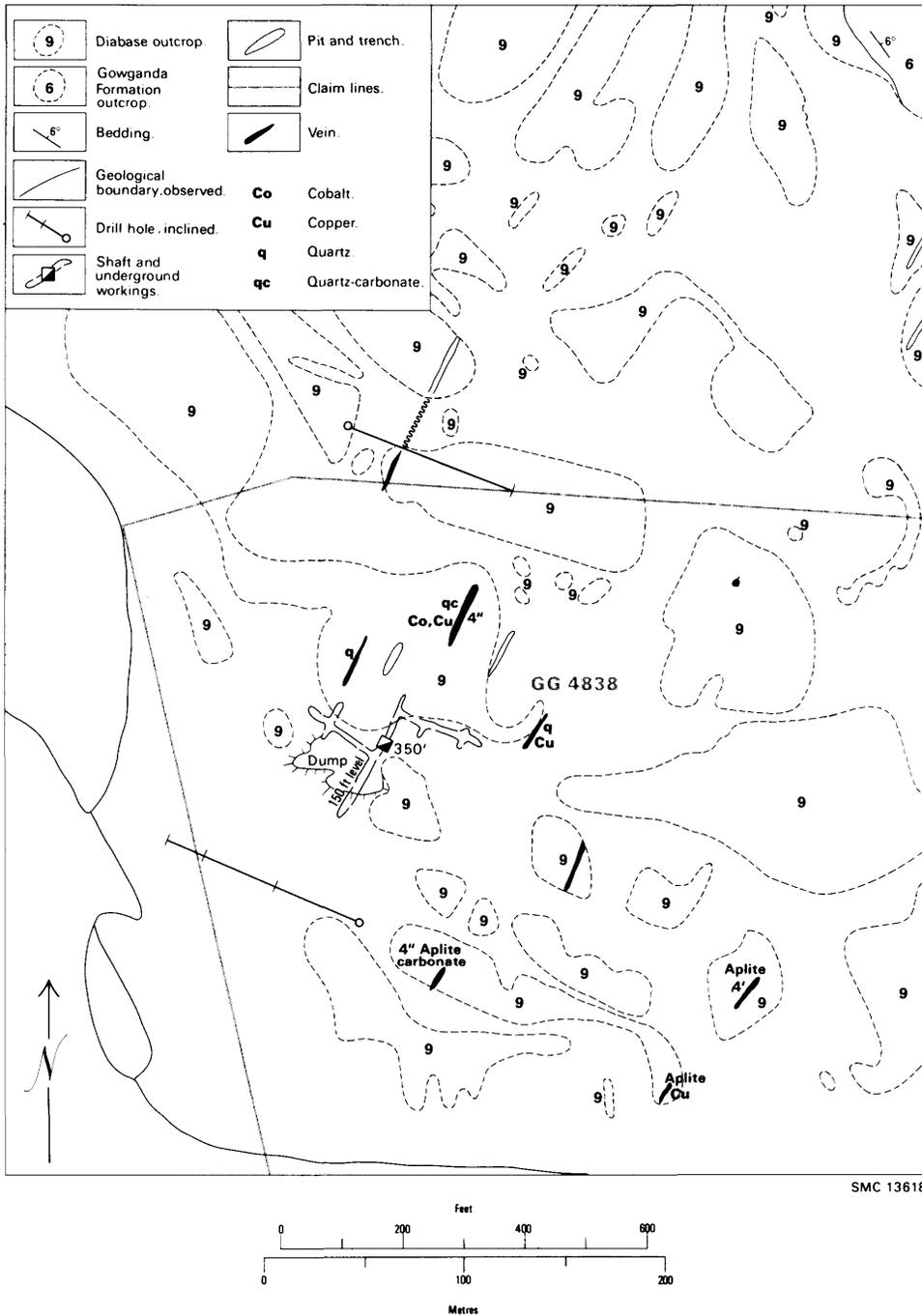
Figure 15—Plans of geology in vicinity of The Haultain (88) shaft, the underground workings in the shaft, and diamond drilling by Roy Silver Mines Limited.
